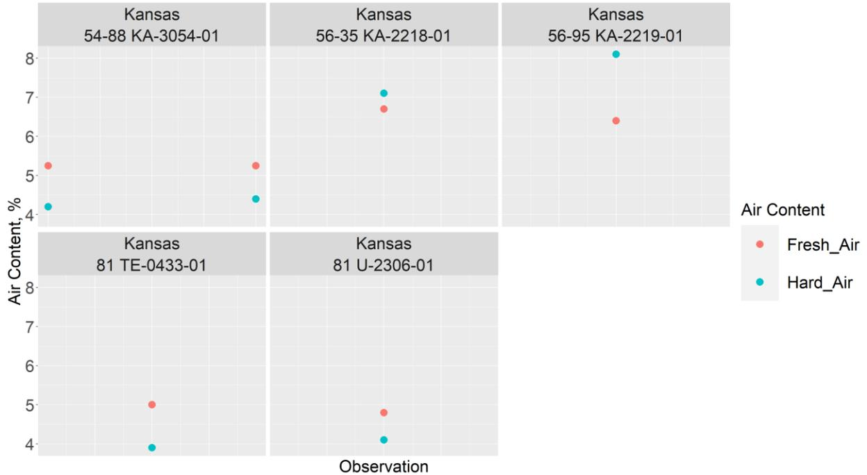
**Figure 51. Fresh and hardened air content**
