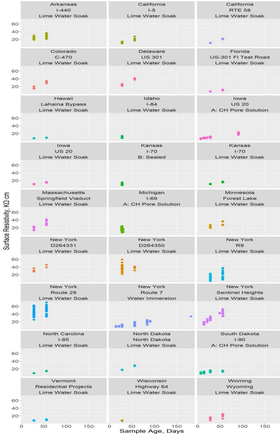
**Figure 68. Surface resistivity versus age for various locations**
