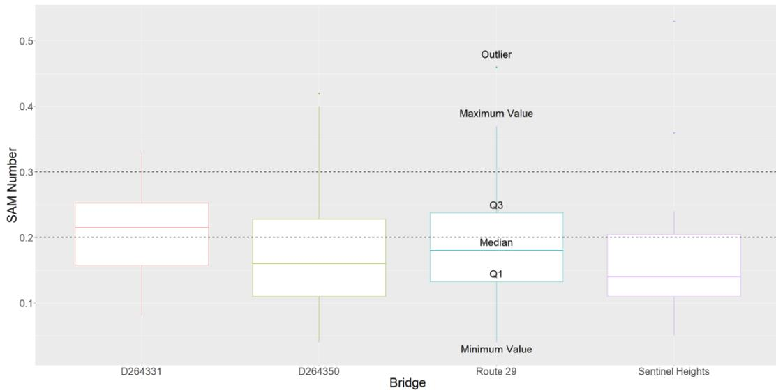
**Figure 40. SAM box and whisker data for bridges**
