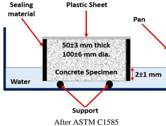
**Figure 4. Specimen setup in ASTM C1585**
