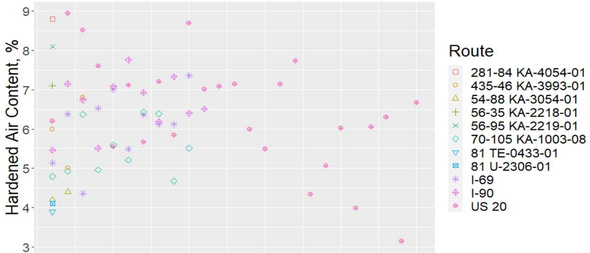
**Figure 57. Scatter data for hardened air content**
