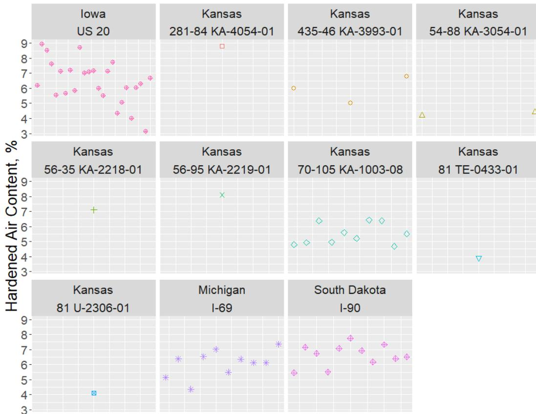
**Figure 58. Hardened air content for various locations**
