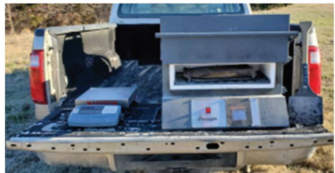
**Figure 5. Phoenix testing device**
