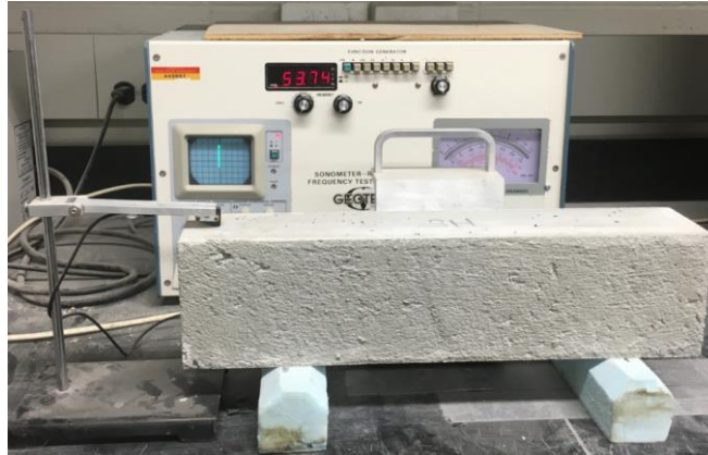
Figure 3.8. Fundamental transverse frequency measurement for dynamic modulus
