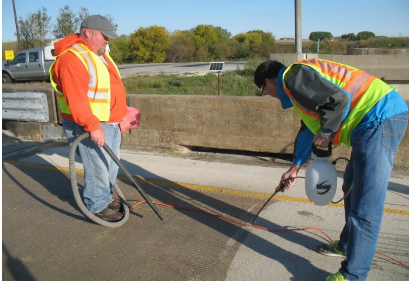
Figure 5.3. Crack survey using wet test method (water used to wet concrete surface)
