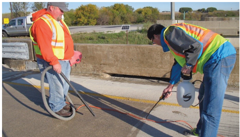
Crack survey being conducted on concrete overlays in the field
