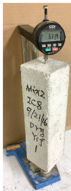
Concrete specimen being tested for free drying shrinkage
