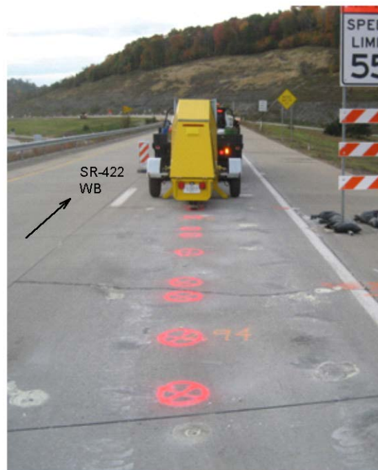
Figure 58. TS7: Photograph showing FWD testing along the center lane
