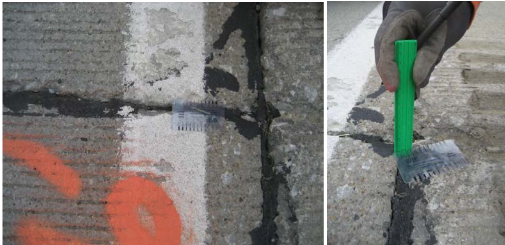
Figure 9. Crack width (left) and fault (right) measurements
