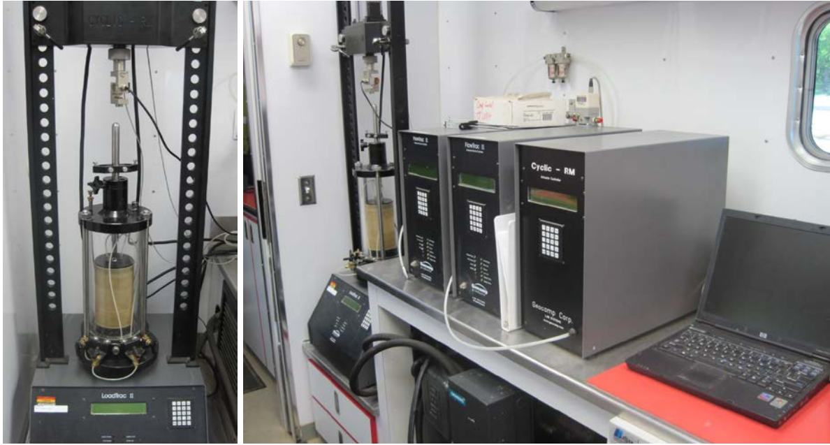
Figure 1. Triaxial chamber and load frame (left) and computer setup (right)
