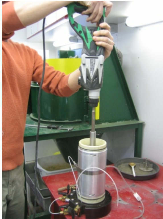
Figure 3. Preparation of an OGS sample for laboratory M_r and UU testing
