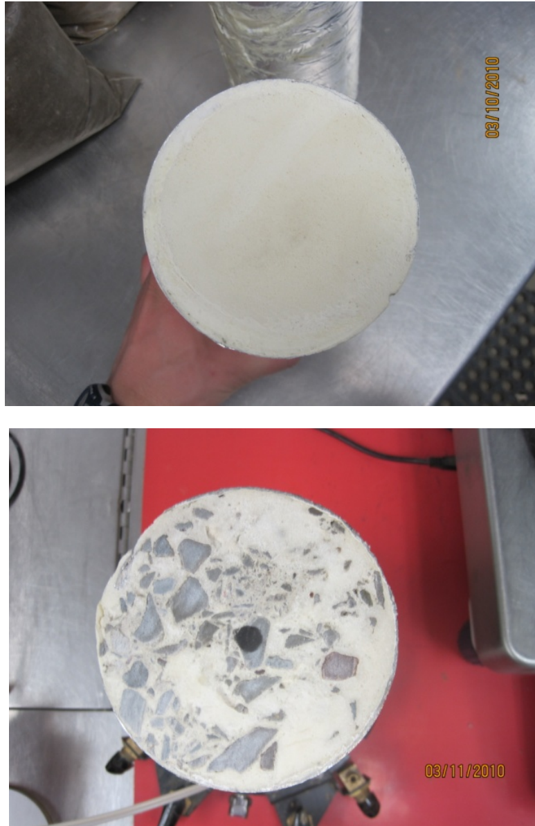
Figure 5. Top view of HDP foam (top) and OGS+Foam mixture (bottom) samples
