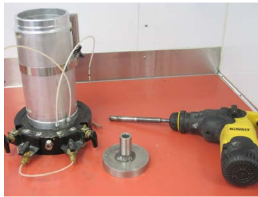
Figure 17. Split mold, steel platen (4 in. diameter), and vibratory hammer for compaction of subbase material samples
