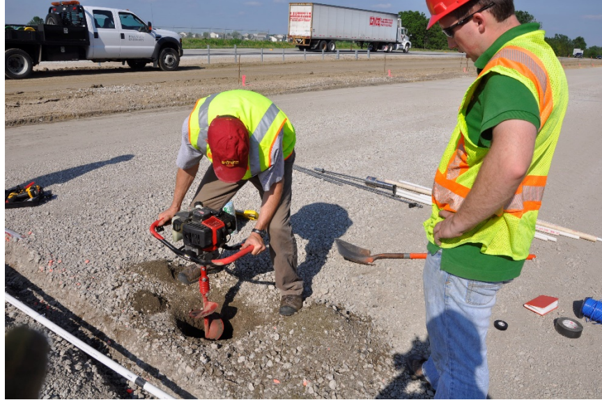
Figure 35. Preparation of a vertical hole to install temperature sensors down to about 1.2 m below surface
