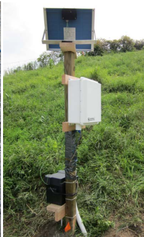
Figure 36. Vertical and horizontal temperature probes (left) and temperature data acquisition setup (right)
