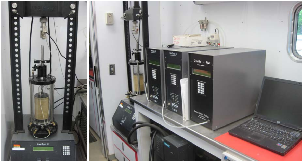
Figure 19. Triaxial chamber (left) and triaxial chamber, load frame, and computer equipment for resilient modulus tests (right)
