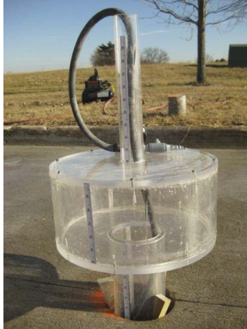
Figure 2. Borehole permeameter setup developed by Iowa State University (Zhang et al. 2013)
