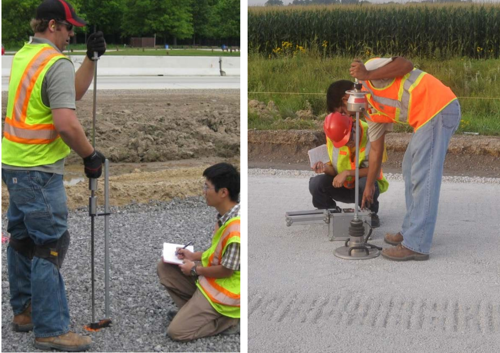
Figure 30. DCP testing (left) and Zorn LWD testing (right)
