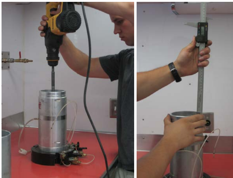
Figure 18. Compaction of subbase material samples in the split mold (left) and verification of thickness of each lift using calipers (right)
