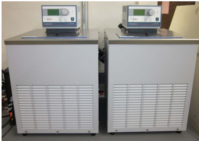
Figure 26. Temperature control water baths used to freeze and thaw samples
