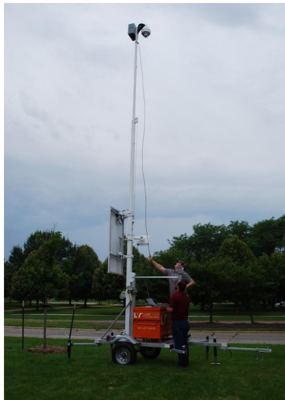
Figure 4-1. Video data collection array
