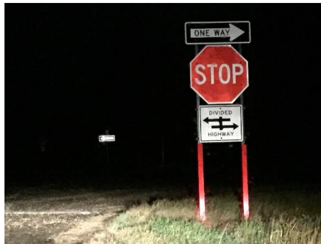
Figure 3-7. Nighttime view of retroreflective strip
