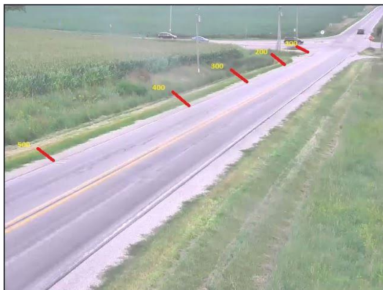
Figure 4-4. Marks placed in video frame to ensure distances are visible to data reductionists
