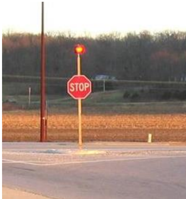
Figure 1-4. Beacon on a stop sign
