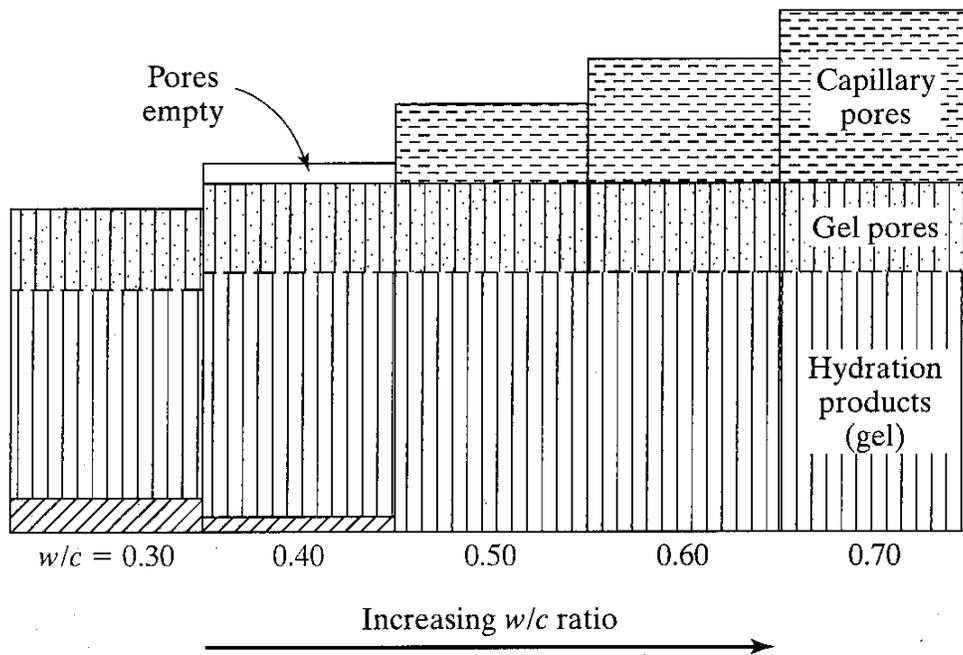
**Figure 2. Relationship between porosity and w/c [8]**
