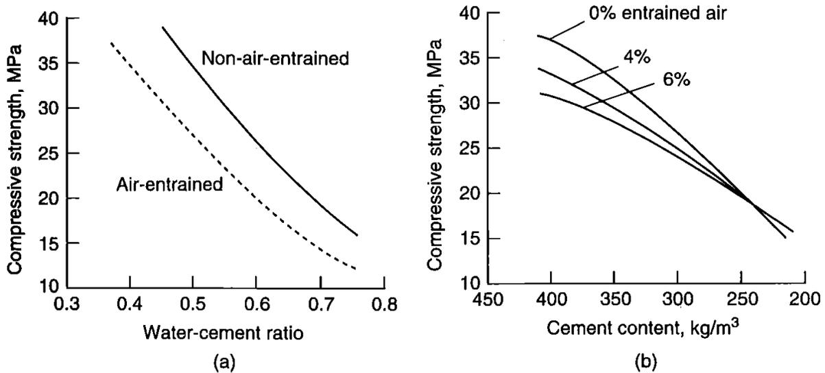
**Figure 4. Influence of entrained air on compressive strength [4]**
