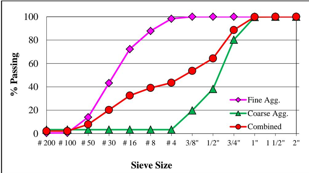
c) ASTM C33 gradation graph
