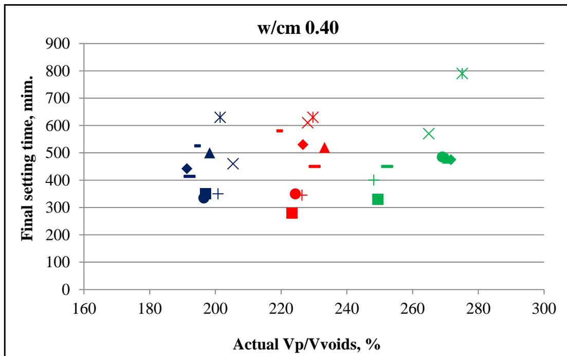
Figure 13. The relationship between  $V_p/V_{\text{voids}}$  and final setting time for a  $w/cm$  of 0.40
