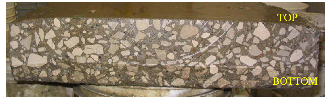
Figure 2.17. Cross-section of pavement slab
