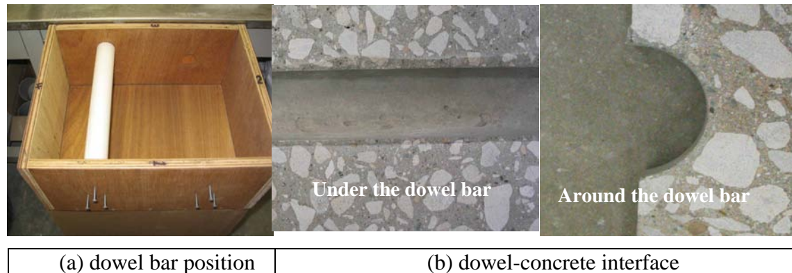
Figure 2.18. Dowel bar test box and concrete slice
