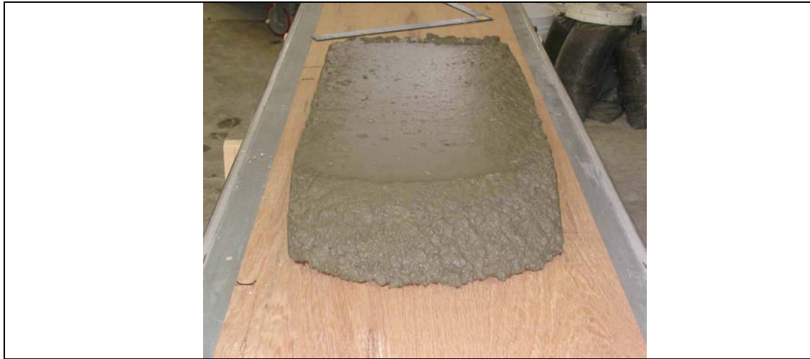
Figure 2.16. Mini-paver test section for SF SCC
