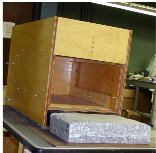
*Mini-paver with section of SCC pavement slab*
