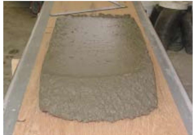
*Test section of SCC extruded from mini-paver*
