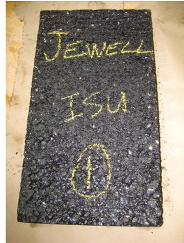
**(b) Thermal conductivity test sample**
