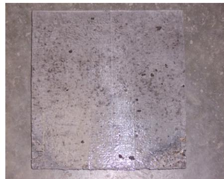
(b) Thermal conductivity test sample
