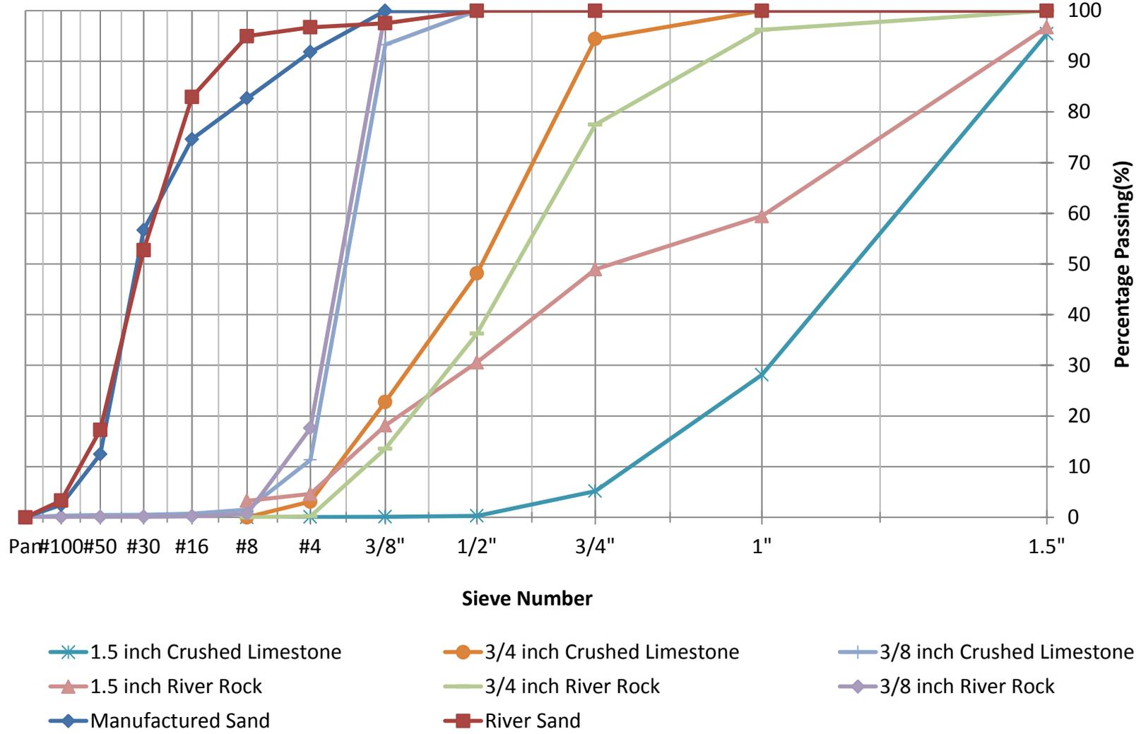
**Figure 2. Sieve analysis for each aggregate type**
