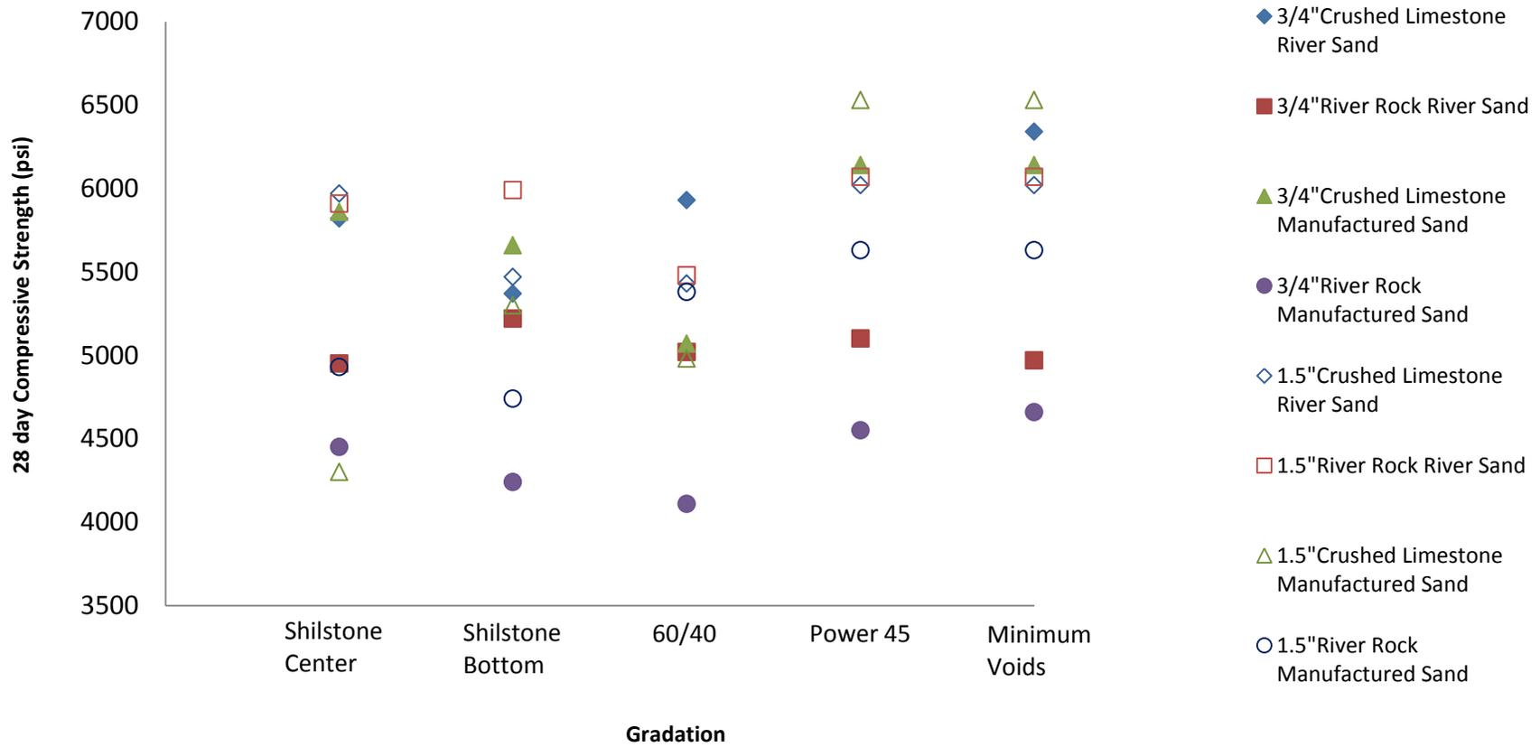
**Figure 27. Gradation compared to the 28-day compressive strength**
