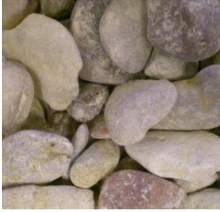
A photograph showing river gravel aggregate. The particles are smooth, rounded, and light-colored, ranging from off-white to light brown. They have a well-rounded angularity.                                           | Combination high and low sphericity with a well-rounded angularity |
