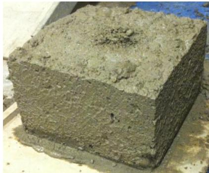
**Figure 15. Mixture passed the box test**
