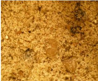
A photograph showing manufactured sand aggregate. The particles are very fine, uniform in size, and light-colored, ranging from off-white to light brown. They are angular with many intermediate particles.            | Angular fines with intermediate particles                          |
