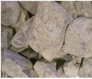
A photograph showing several pieces of crushed limestone aggregate. The particles are light-colored, ranging from off-white to light grey, and have a mid-angular shape with some sharp edges and some smoother surfaces. | Combination of low and high sphericity with a mid-angularity       |
