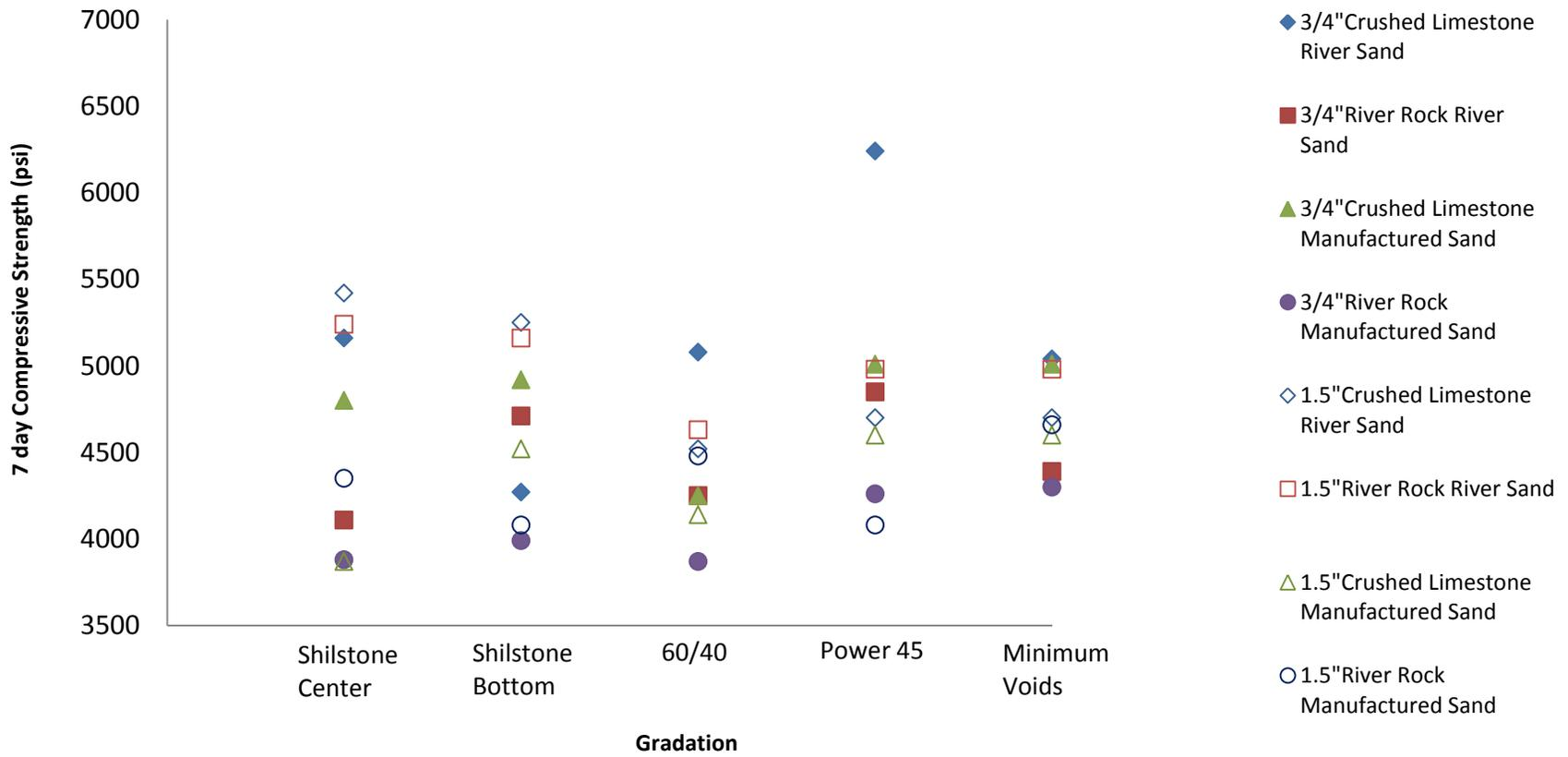
**Figure 26. Gradation compared to the 7-day compressive strength**
