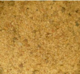
A photograph showing river sand aggregate. The particles are very fine, uniform in size, and light-colored, ranging from off-white to light brown. They are mostly spherical with very few intermediate particles.      | Fines with very few intermediate particles                         |
