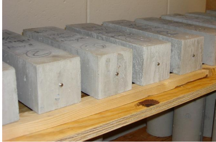
Figure 32. Drying shrinkage samples
