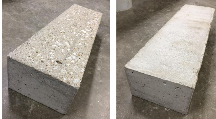
Figure 20. Slab surfaces: sandblasted surface (left) and troweled surface without sandblasting (right)
