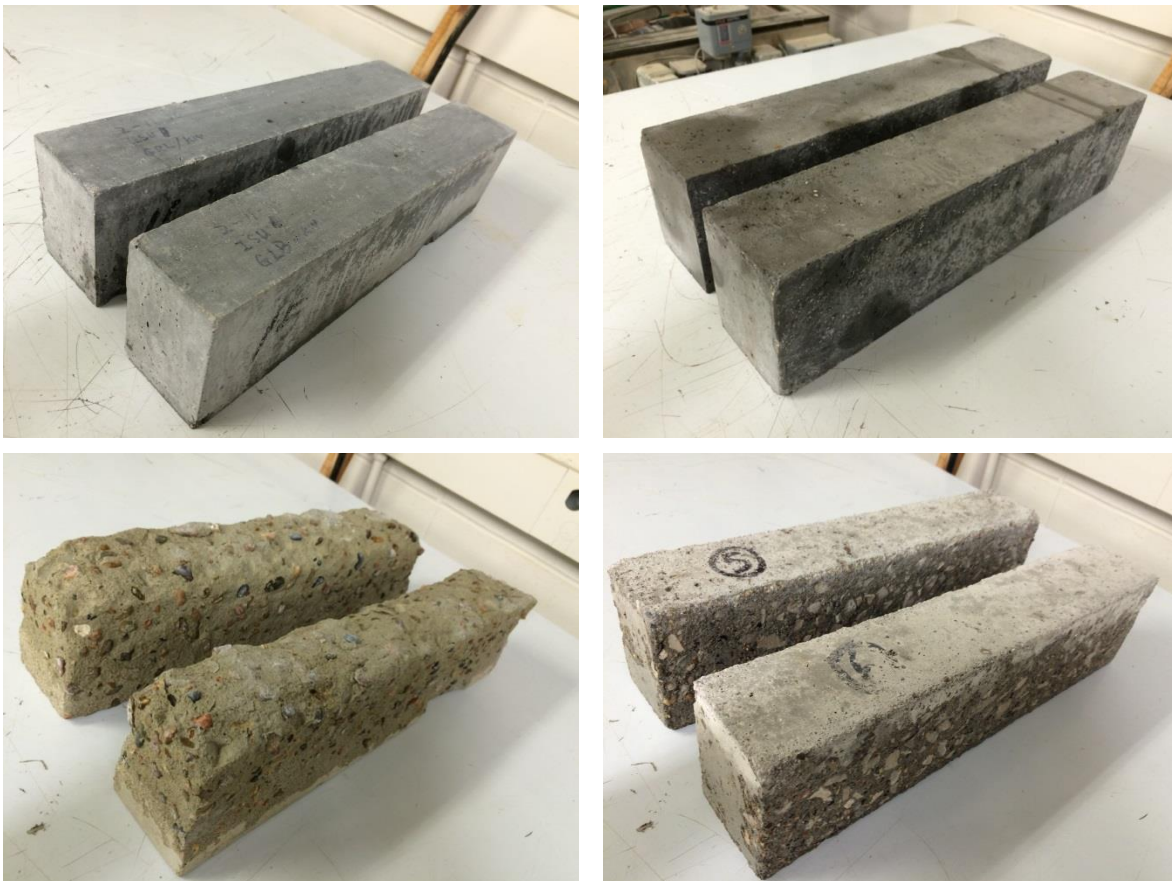
Figure 29. Prisms after 300 F-T cycles: HPM (upper left), HPM-f (upper right), RSC (lower left), and C-3WR-C20 (lower right)
