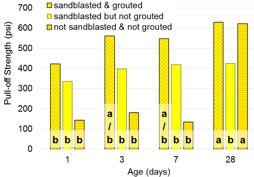
Figure 26. Pull-off strength of rapid repair mixtures with O-4WR substrates showing (a) substrate failure and (b) bond failure
