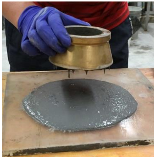
Figure 7. Flow of rapid repair mixture
