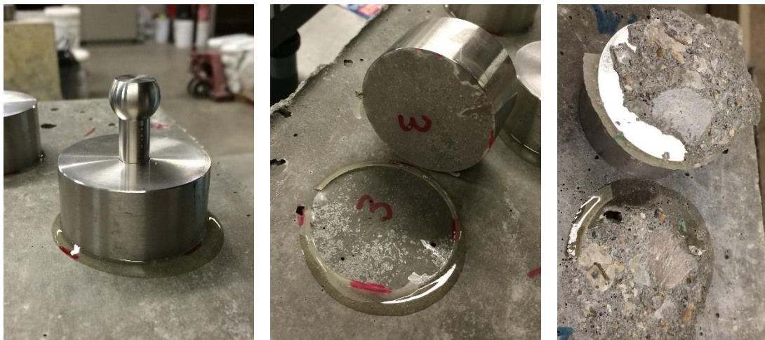
Figure 23. Testing of epoxy: steel disk epoxied to an uncut concrete surface (left), epoxy failure after direct-pull off test (center), and concrete failure due to good epoxy bond (right)
