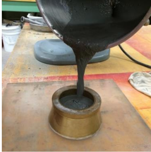
Figure 6. Filling of mold with rapid repair mixture
