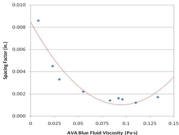
*Effect of blue fluid viscosity on AVA measurements*
