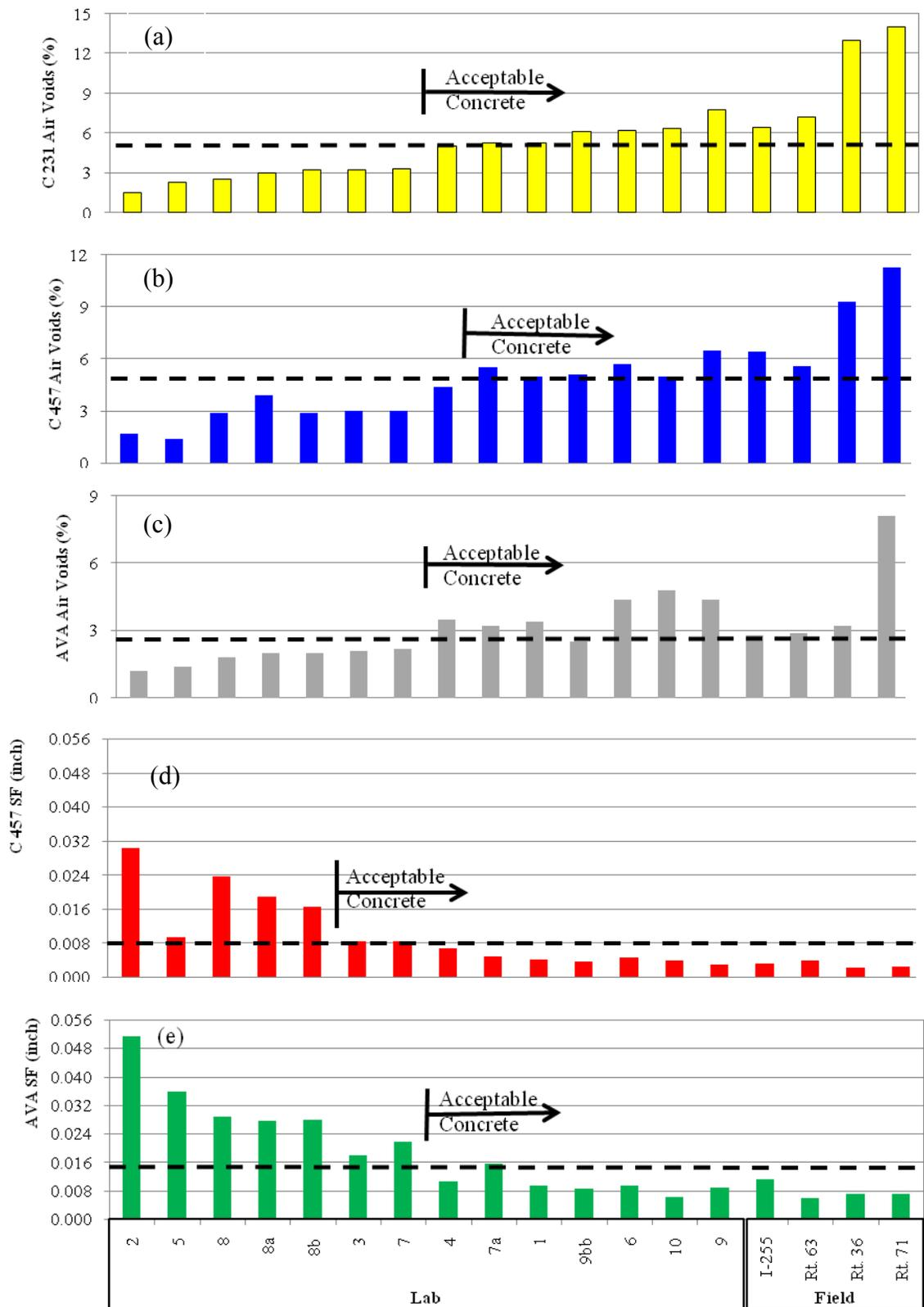
Figure 20. Missouri data—acceptance criteria for total air voids and spacing factors
