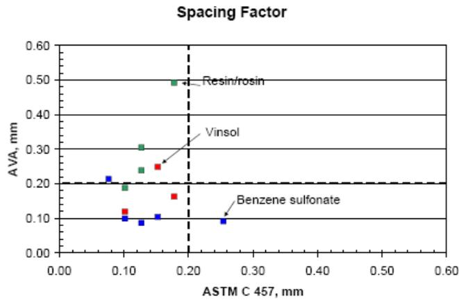
Figure 14. CTLGroup study—acceptance/rejection agreement in spacing factors measured by AVA and C457 (Acceptance criteria: spacing factor  $\leq 0.008$  in.)
