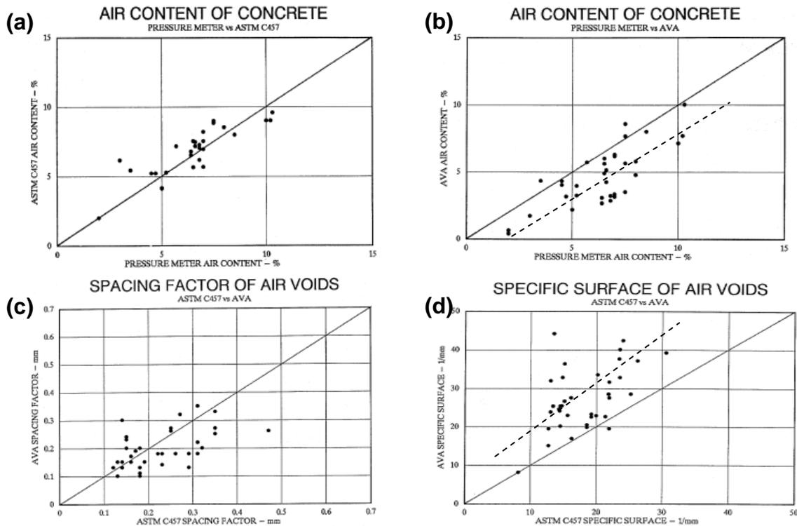
**Figure 3. FHWA study on AVA—relationships between results from different test methods (a) C457 and C231 air contents; (b) AVA and C231 air contents; (c) AVA and C457 spacing factors; and (d) AVA and C457 specific surfaces**
