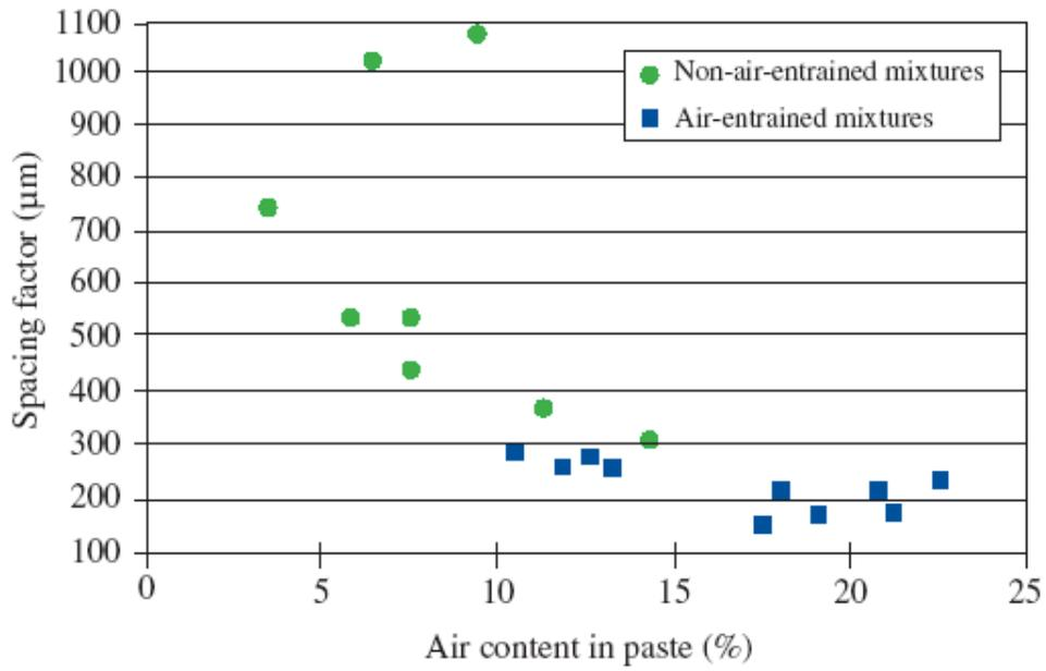
Figure 8. Spacing factor versus air content in paste
