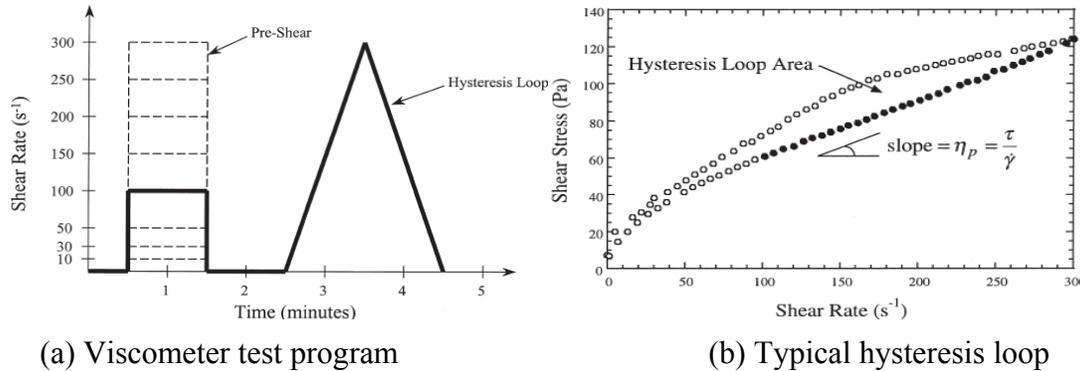
**Figure 37. Rheometer experimental program (Williams et al. 1999)**
