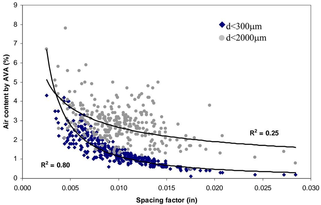
Figure 9. MCO study—relationship between AVA air content, bubble size, and spacing factor
