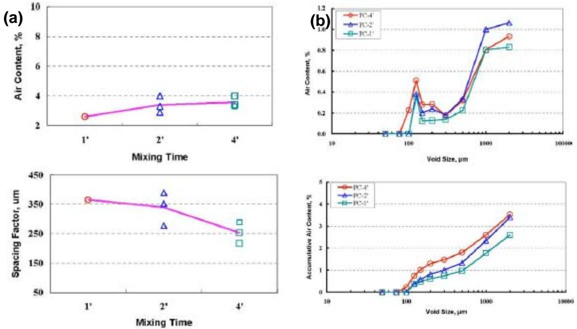
Figure 12. Other ISU study—effect of mixing time on AVA measurements (a) on air content and spacing factor (b) on void size distribution
