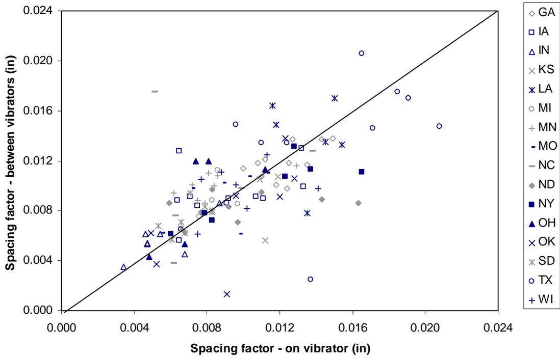
**Figure 6. MCO study—spacing factors of samples between vibrators versus those on vibrators**
