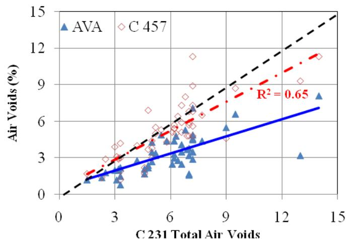
**Figure 29. Statistical analysis—total air content measured by different test methods**
