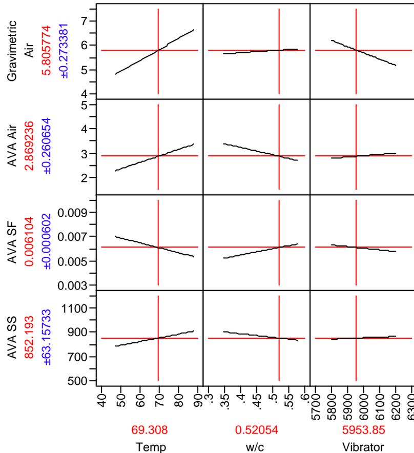
**Figure 35. Statistical analysis—effects of ambient temperature, concrete w/cm, and vibrator energy effect**
