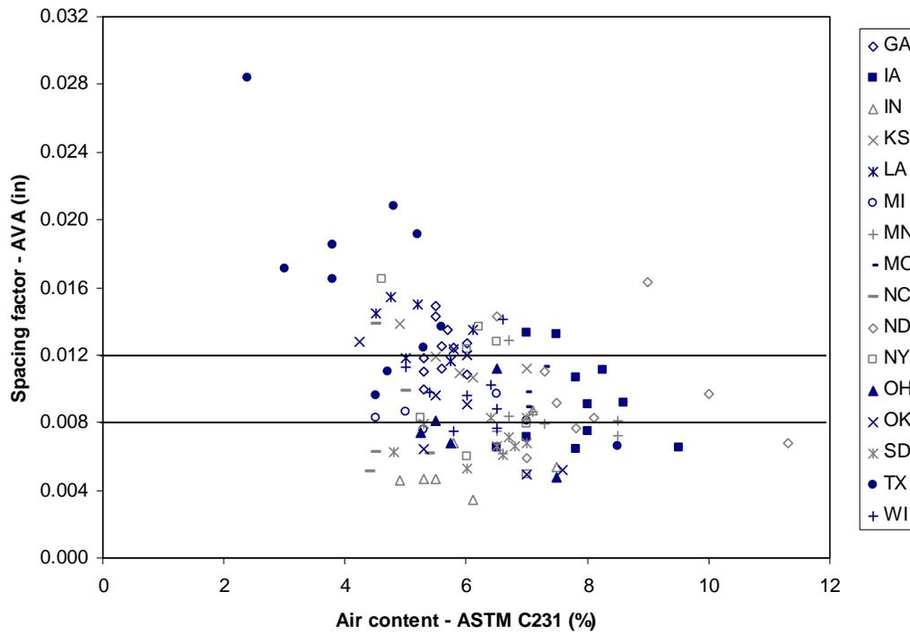
**Figure 7. MCO study—spacing factor versus total air content**
