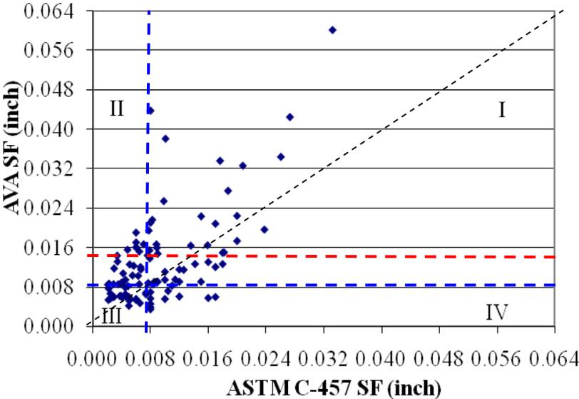
**Figure 31. Statistical analysis—relationship between spacing factors measured by AVA and C457**
