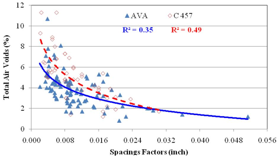
**Figure 30. Statistical analysis—relationship between AVA total air and spacing factor**
