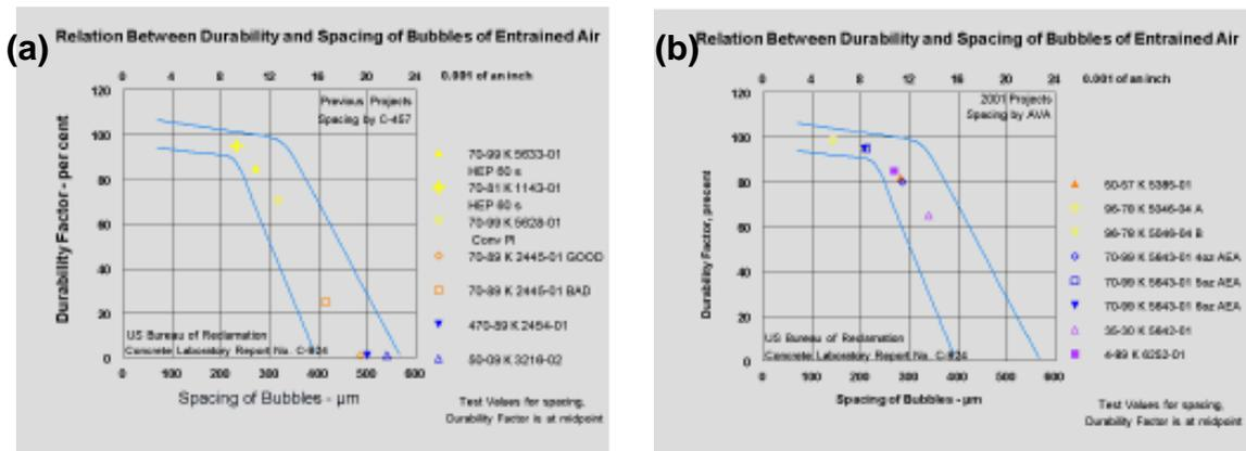
**Figure 4. Kansas study—correlation of durability factor and spacing factor (a) C457 spacing factor and (b) AVA spacing factor**
