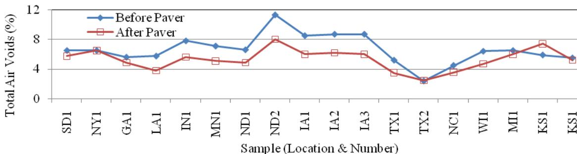
**Figure 33. Statistical analysis—effect of sampling locations on C231 air content measurements**
