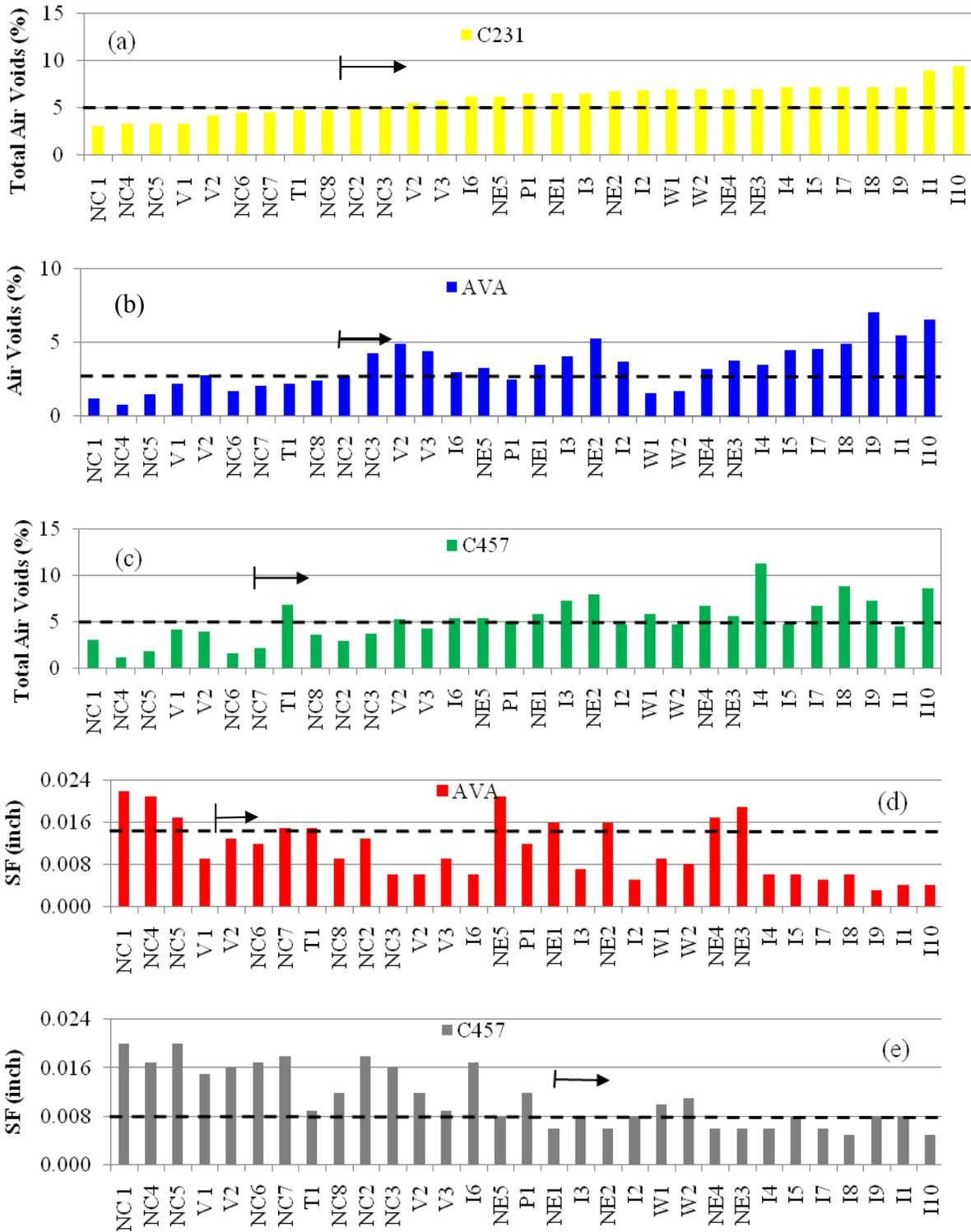
Figure 24. FHWA Mobile Lab—acceptance criteria for total air voids and spacing factors
