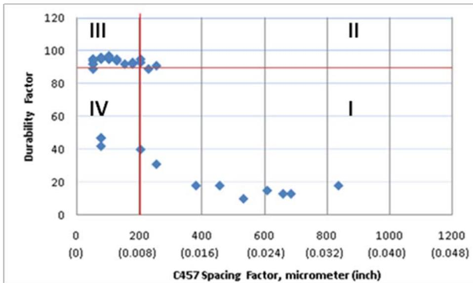
(b) Spacing factor measured from C457
