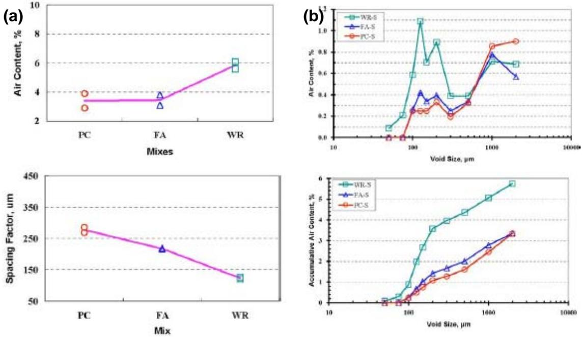
Figure 11. Other ISU study—effect of concrete materials on AVA measurements (a) air content and spacing factor (b) void size
