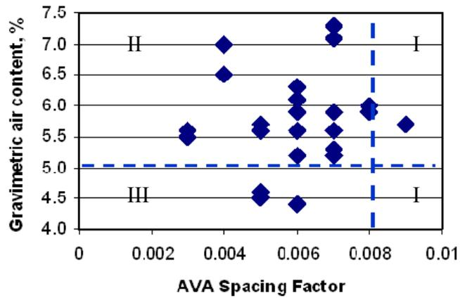
Figure 26. Michigan results—acceptance/rejection agreement between AVA spacing factor ( $\leq 0.008$  in.) and gravimetric air content ( $\geq 5.0\%$ )
