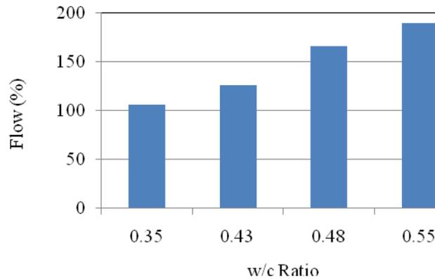
**Figure 38. Effect of different w/c on flowability**
