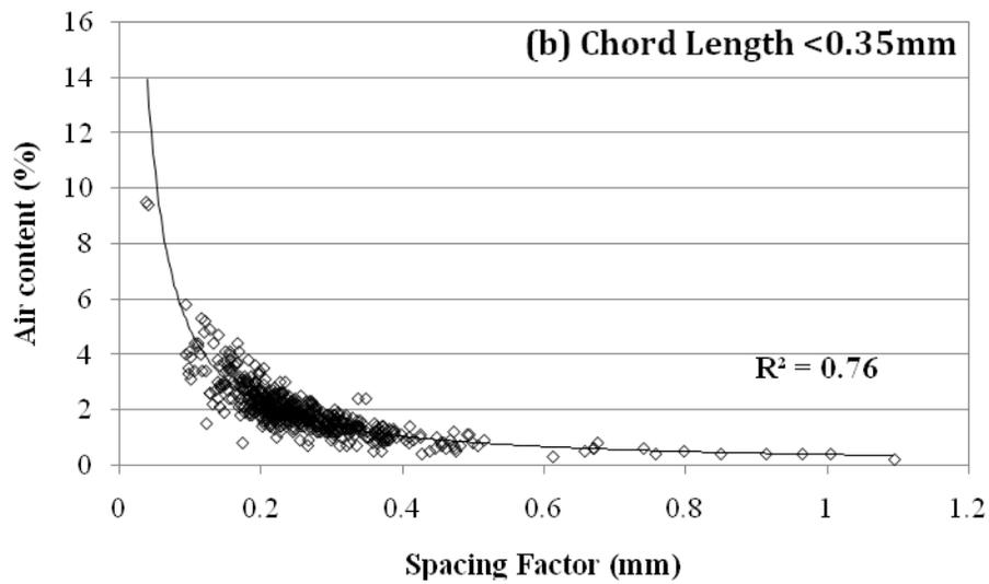
**Figure 28. Kansas DOT data—relationship between AVA spacing factor and air content max bubble size (a) large (b) small**
