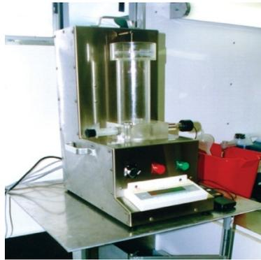
**Figure 2. Air-void analyzer**
