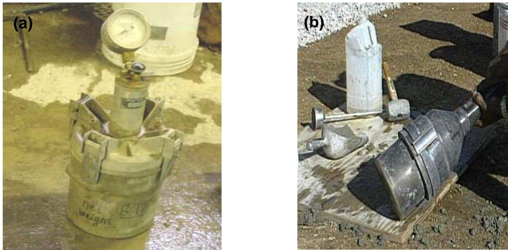
**Figure 1. Devices for air content measurement of fresh concrete—(a) ASTM C231 and (b) ASTM C173**
