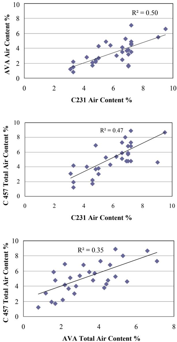
**Figure 21. FHWA Mobile Lab results—air content measured with different test methods**
