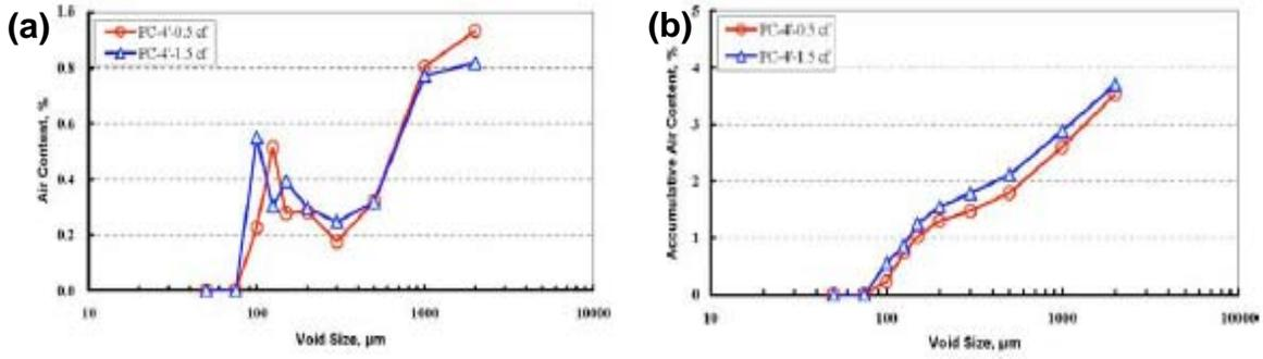
Figure 13. Other ISU study—effect of mixer on AVA measurements (a) on total air content and (b) on accumulative air content
