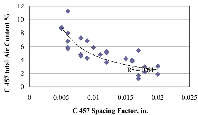
**Figure 22. FHWA Mobile Lab results—relationship between air content and spacing factor obtained from different test methods**
