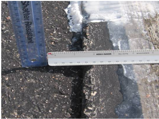
(c) Lane to shoulder drop-off at slab #6
