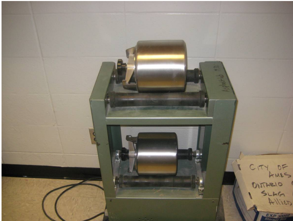
Figure 7. Micro-Deval testing machine in PCC laboratory, Iowa State University
