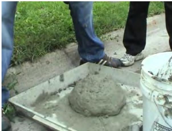
**Figure 6–14. Slump of S4TH-M2**
