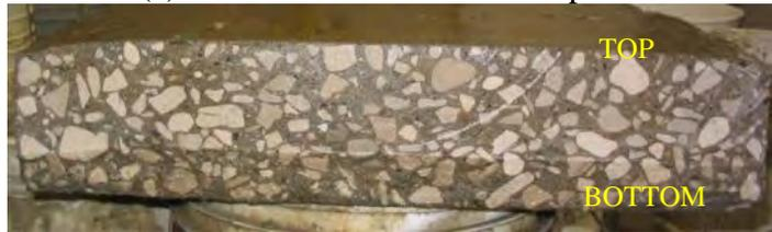
(b) Cross section of the above concrete slab
