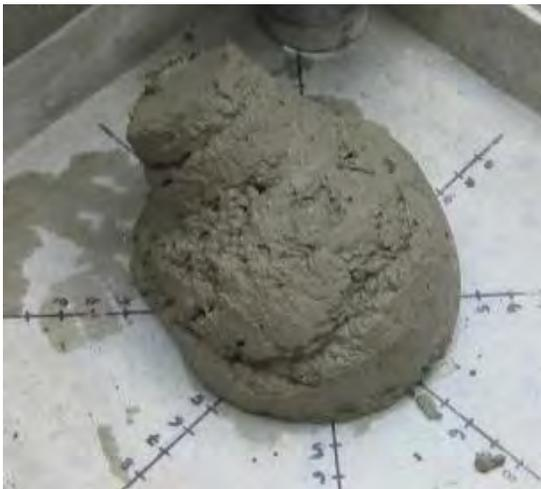
**Figure 6-25. Initial slump of NR-M1-A**
