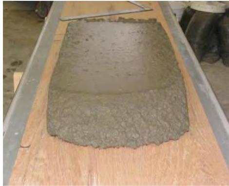
(a) Concrete slab from a mini-paver test
