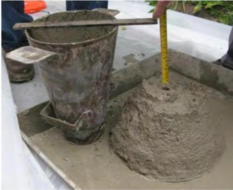
**Figure 6-27. Slump of NR-M2-A**
