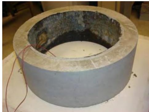
Cracked concrete ring
