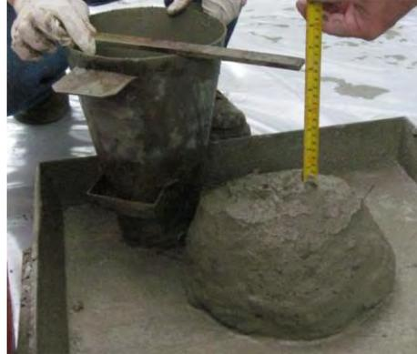
**Figure 6-28. Slump of NR-M3-A**
