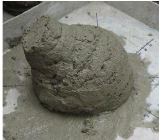
**Figure 6-26. Slump of NR-M1-A after addition of HRWR and water**
