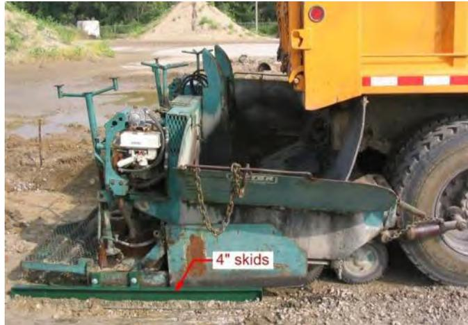
**Figure 6–2. Asphalt paver used for slip-form paving**
