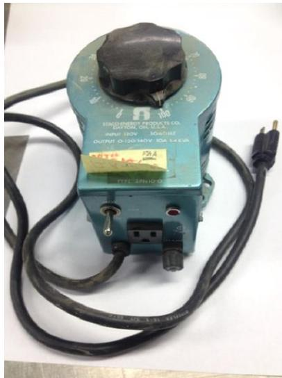
**Figure 4. Variable transformer**
