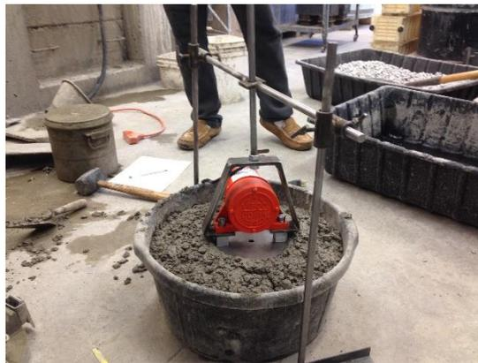
**Figure 6. Completed VKelly test**
