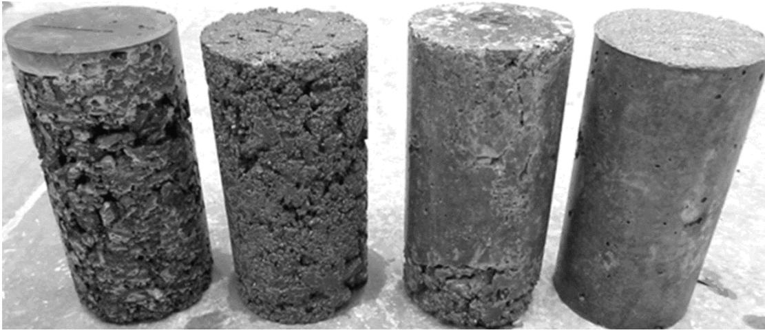
**Figure 4. Cylinders made with mixtures with increasing cementitious content from 400 to 700 lb./yd.<sup>3</sup>**
