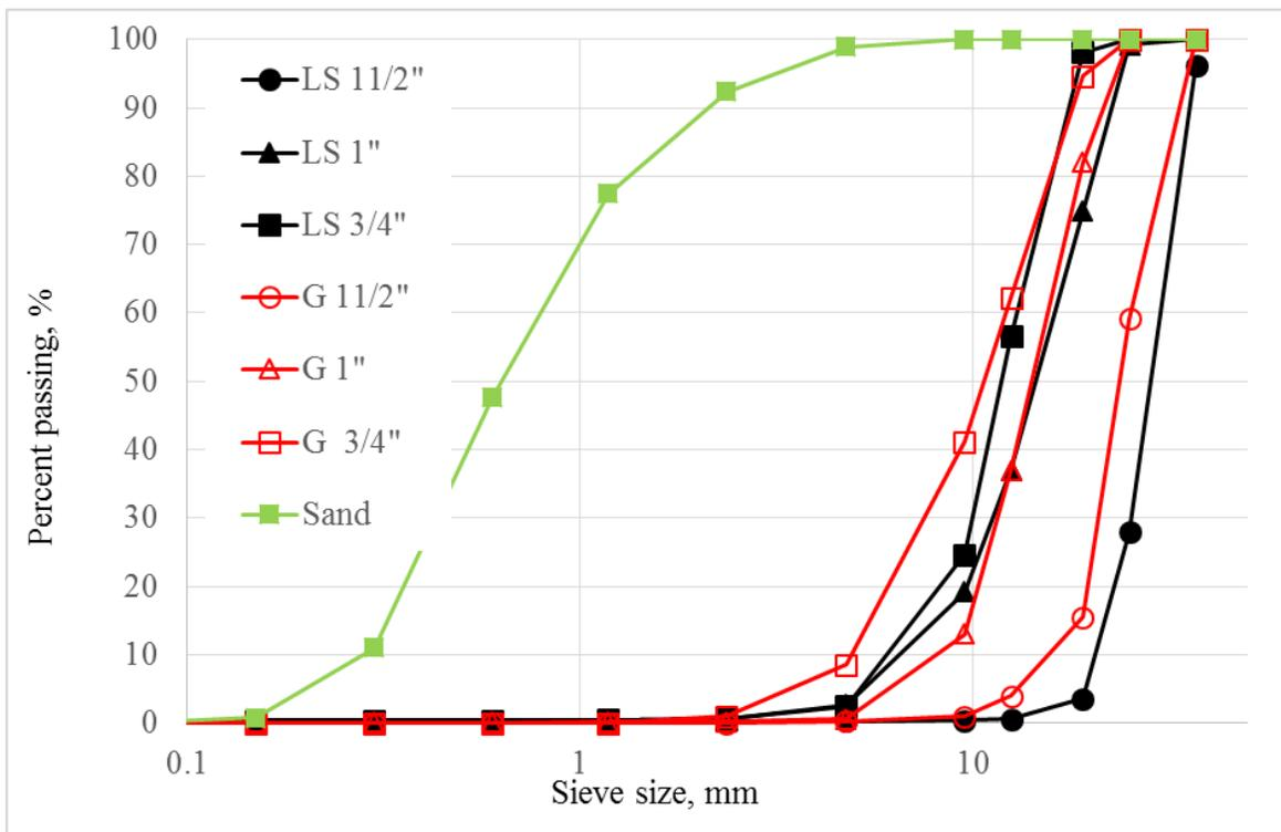
**Figure 10. Gradations of coarse and fine aggregate**
