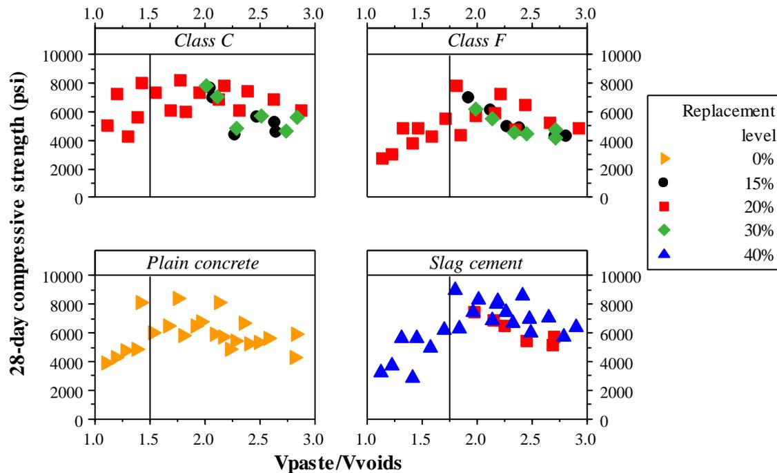
**Figure 7. Required paste system for 28-day compressive strength**
