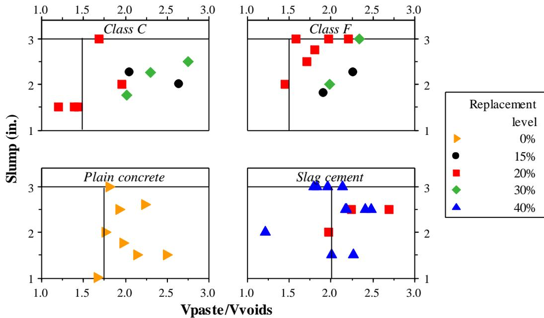
**Figure 3. Required paste system for workability**
