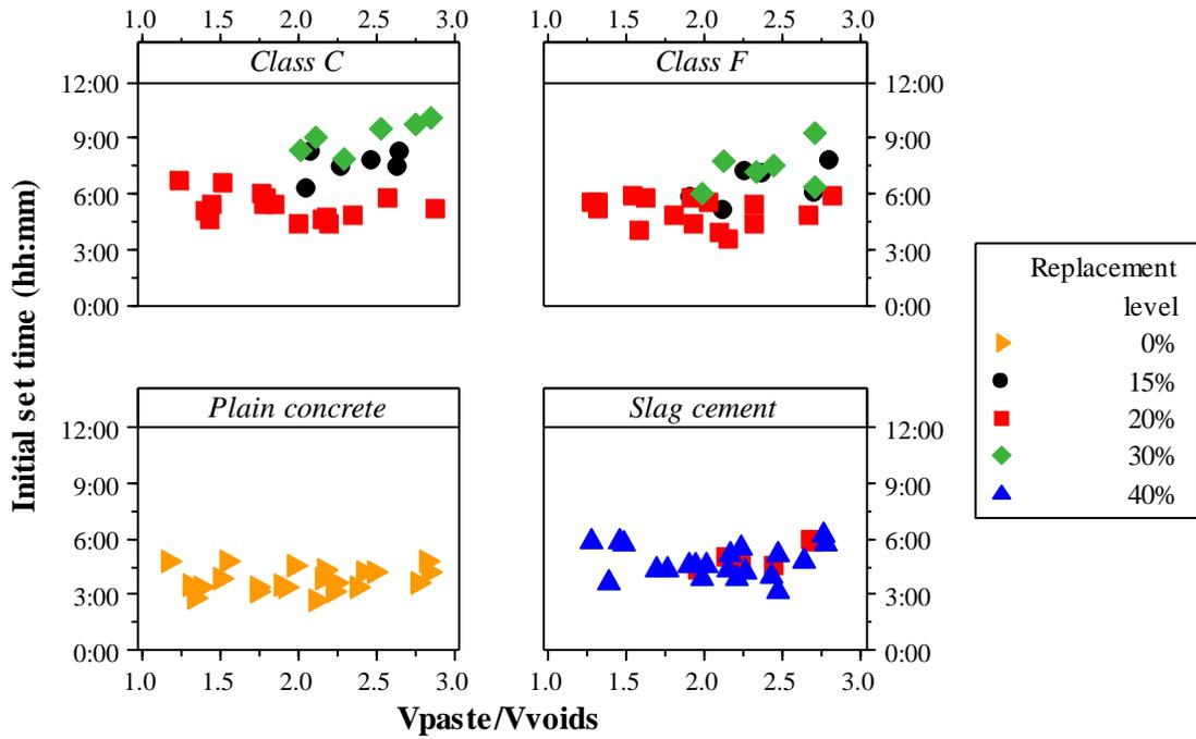
Figure 5. Required paste system for initial set time
