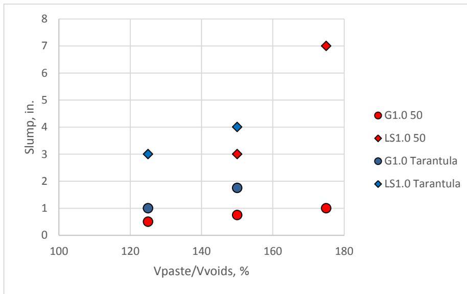
**Figure 11. Slump versus  $V_{paste}/V_{voids}$**
