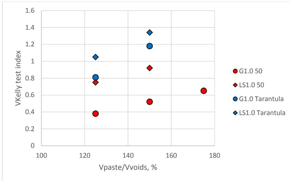
**Figure 12. VKelly test index versus  $V_{paste}/V_{voids}$**
