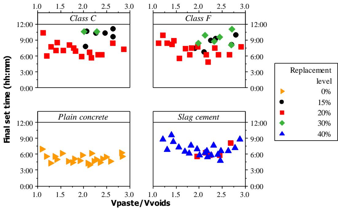
Figure 6. Required paste system for final set time
