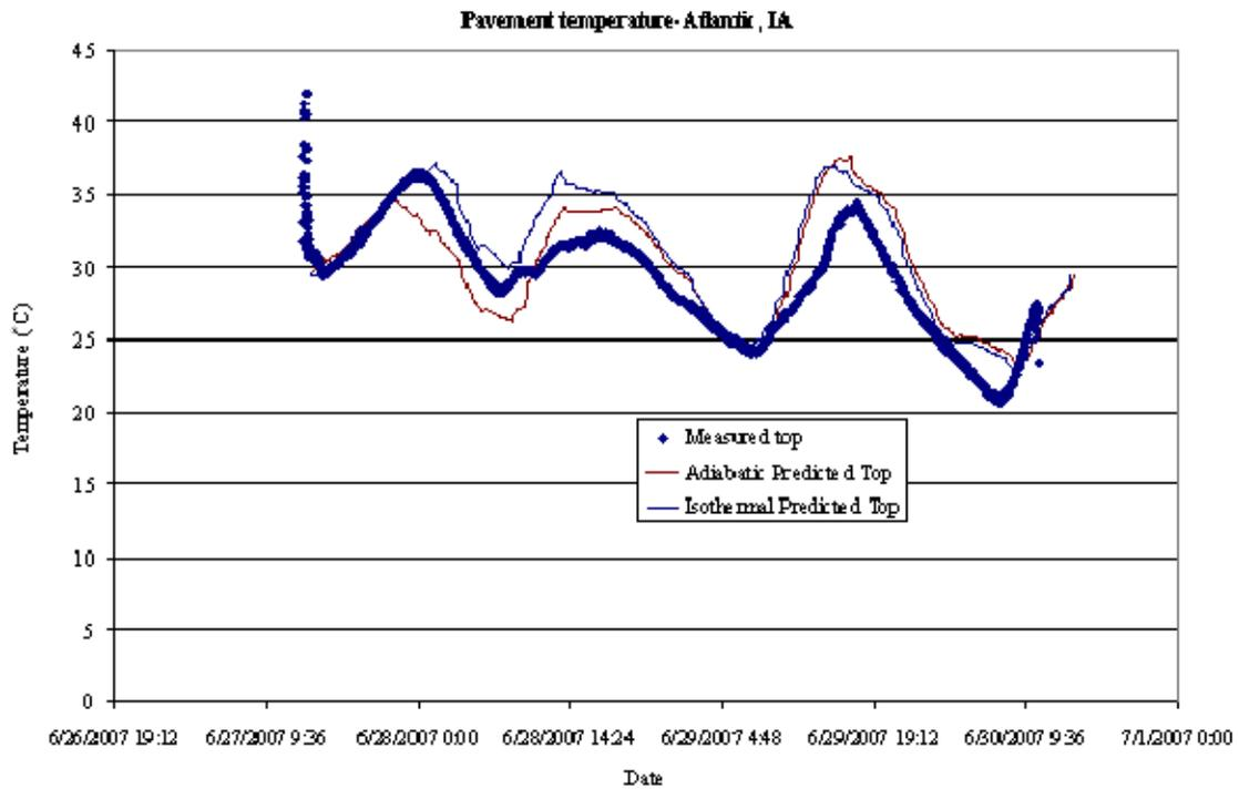
**Figure 104. Predicted pavement temperatures versus measurements (pavement top, Atlantic, IA)**
