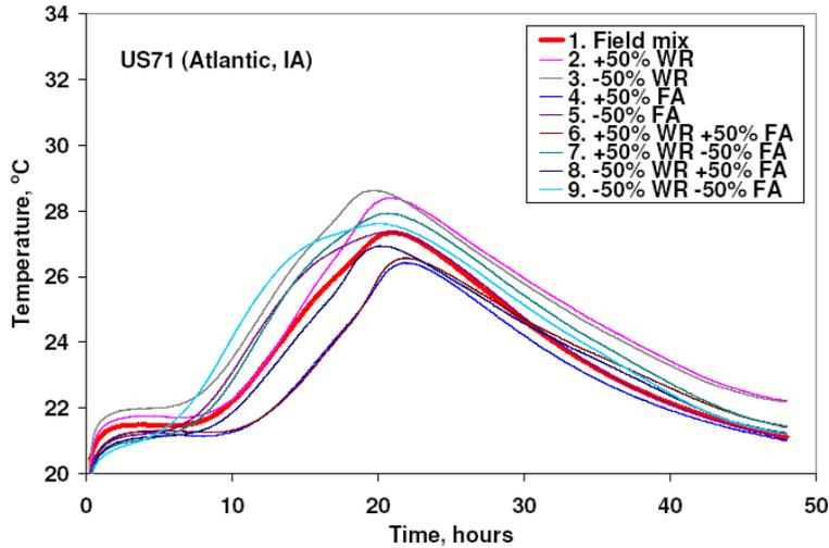
**Figure 30. AdiaCal robust test results of US 71 (Atlantic, IA) concrete mixes**
