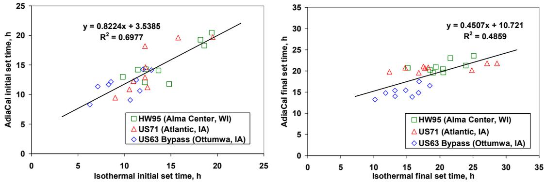
Figure 64. Comparison of isothermal and AdiaCal set time results
