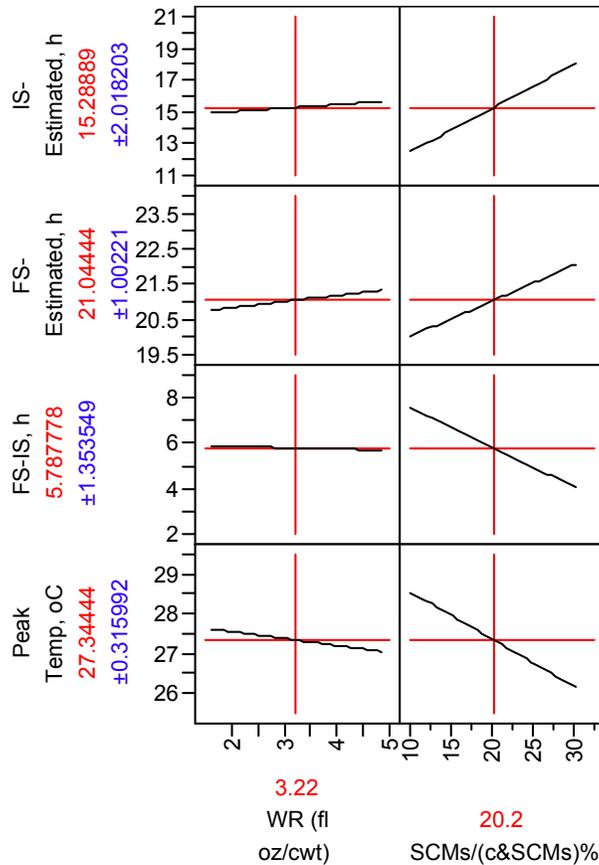
**Figure 43. Statistical analysis from the HW 95 (Alma Center, WI) AdiaCal robust test**
