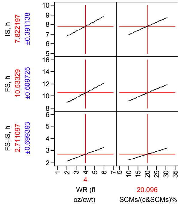
**Figure 61. Effect of mix design on ASTM setting time US63 bypass (Ottumwa, IA) mixes**
