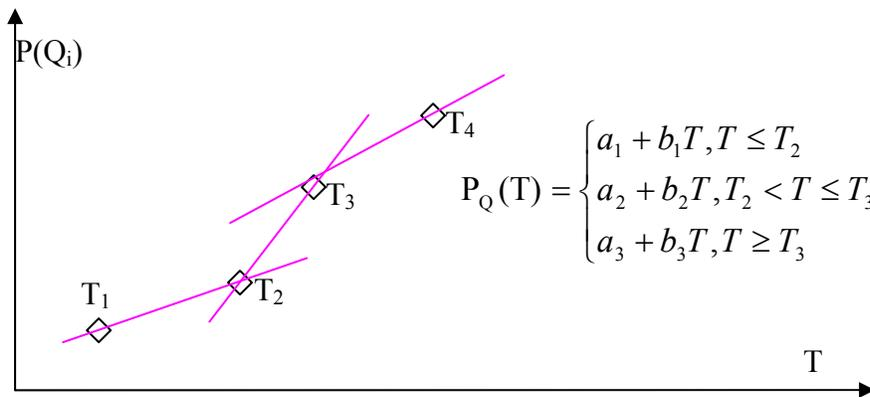
Figure 88. Approximate P vs. T at any heat (Q) state
