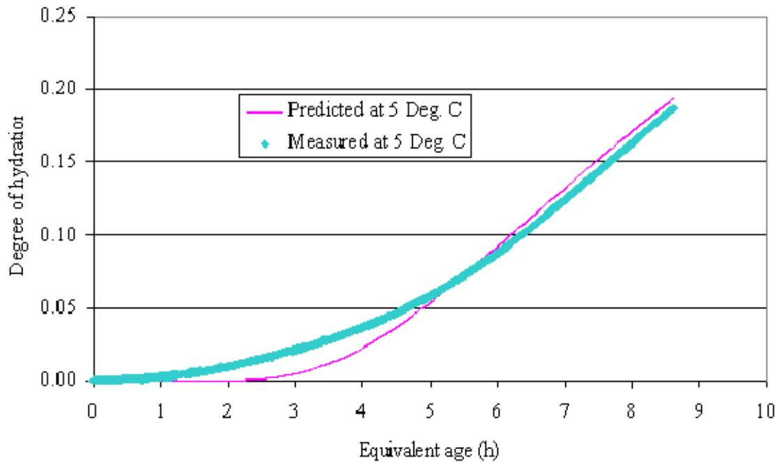
**Figure 77. Predicted degree of hydration vs. measurements at 5 °C (Sample 5, Alma Center)**
