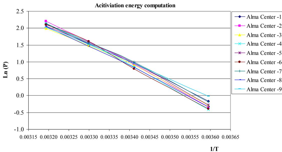
**Figure 68. Activation energy calculation for AlmaCenter site (nine mixes, at four temperatures: 5 °C, 20 °C, 30 °C, and 40°C; P unit: mW/g; T unit: K).**
