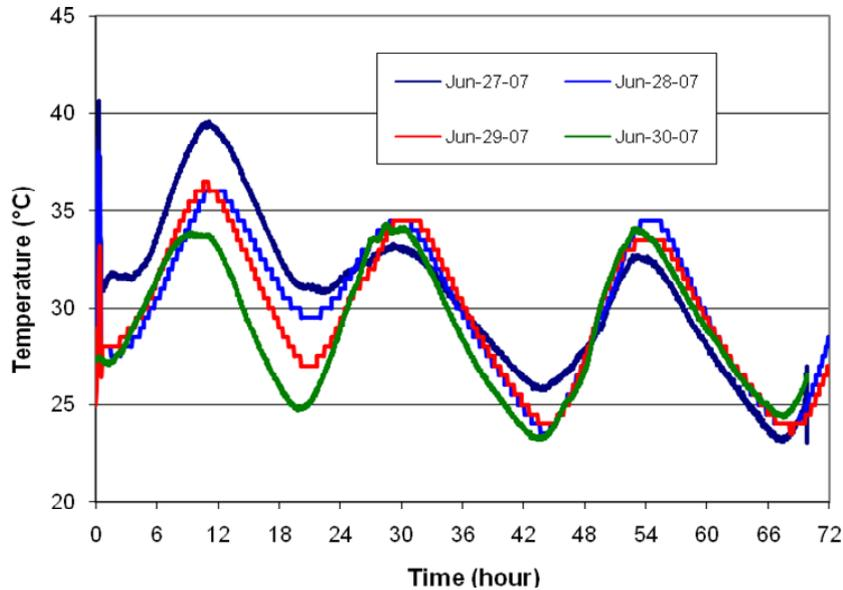
**Figure 13. Pavement temperature from US 71 (Atlantic, IA) measured at the middle on different date**
