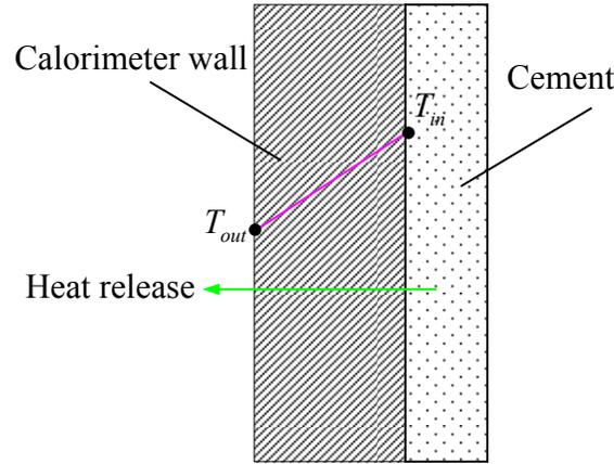
**Figure 89. Heat conduction in the calorimeter wall**
