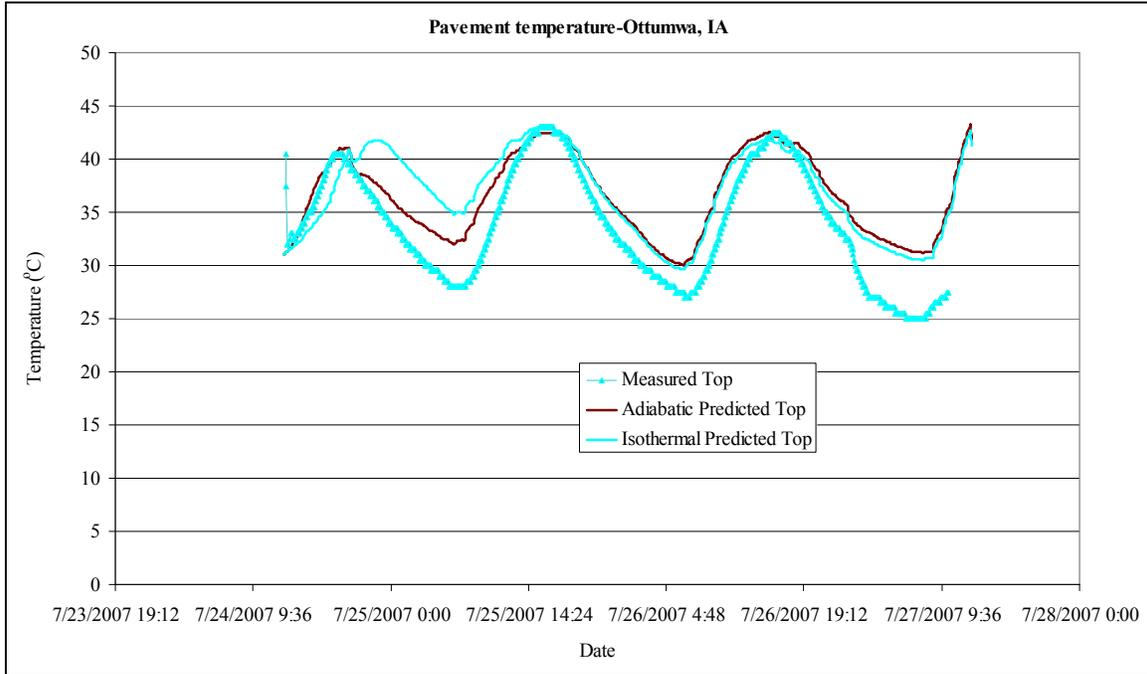
**Figure 110. Predicted pavement temperatures versus measurements (pavement top, Ottumwa, IA)**
