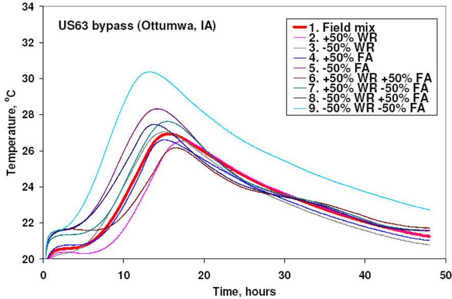
**Figure 51. AdiaCal robust test results of US 63 bypass (Ottumwa, IA) concrete mixes**
