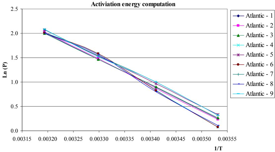
**Figure 69. Activation energy calculation for Atlantic site (nine mixes, at four temperatures: 10 °C, 20 °C, 30 °C, and 40 °C; P unit: mW/g; T unit: K).**
