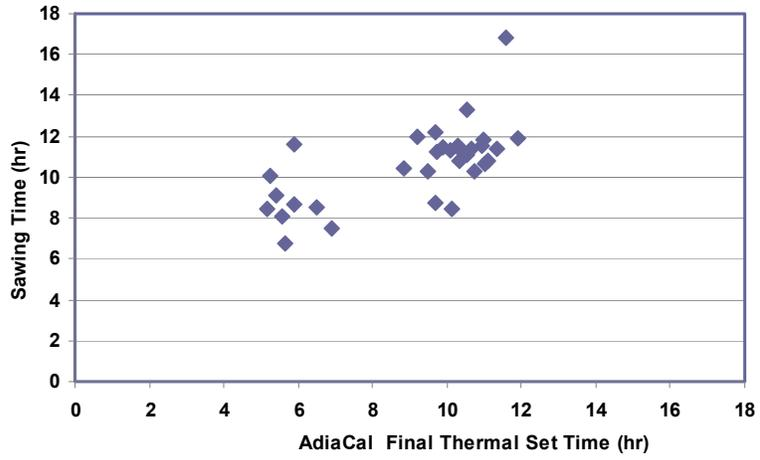
**Figure 29. Pavement sawing time vs. AdiaCal thermal final set time**
