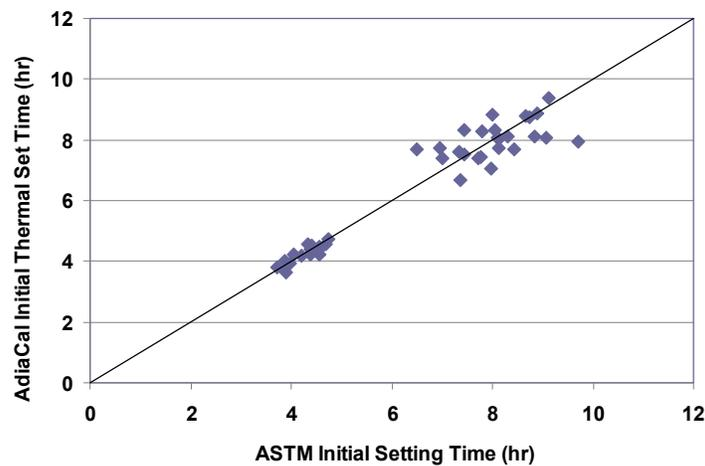
**Figure 26. ASTM set time vs. AdiaCal thermal set time—initial set**
