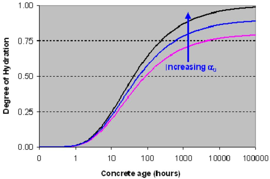
Figure 72. Influence of hydration curve parameter  $\alpha_u$  on degree of hydration
