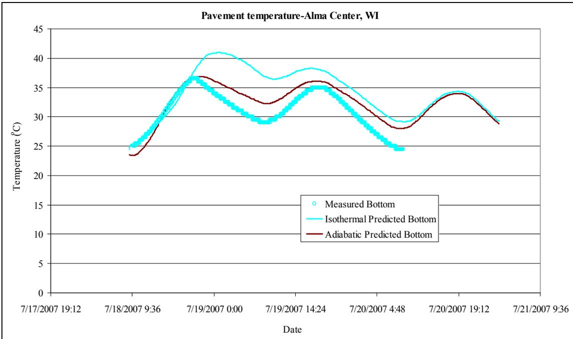
**Figure 100. Predicted pavement temperatures versus measurements (pavement bottom, Alma Center, WI)**
