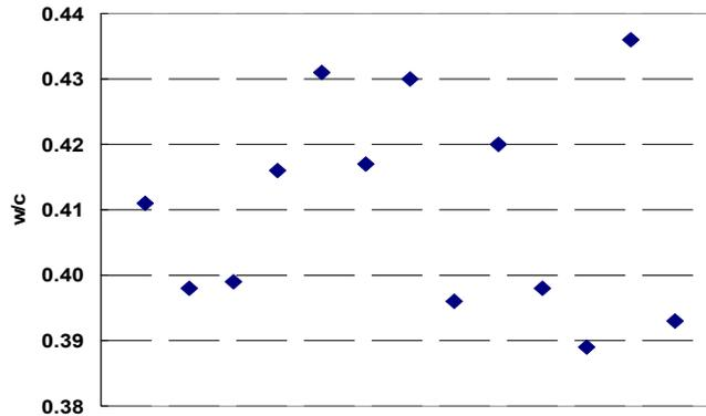
**Figure 4. Water to cement ratio for the mixes of US 71 (Atlantic project)**
