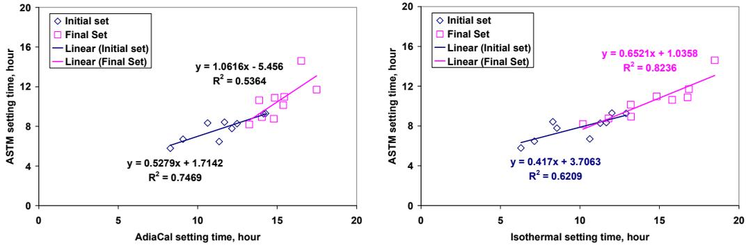
Figure 65. Comparison of ASTM and thermal set time results
