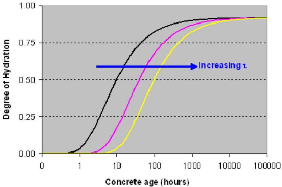
Figure 73. Influence of hydration curve parameter  $\beta$  on degree of hydration
