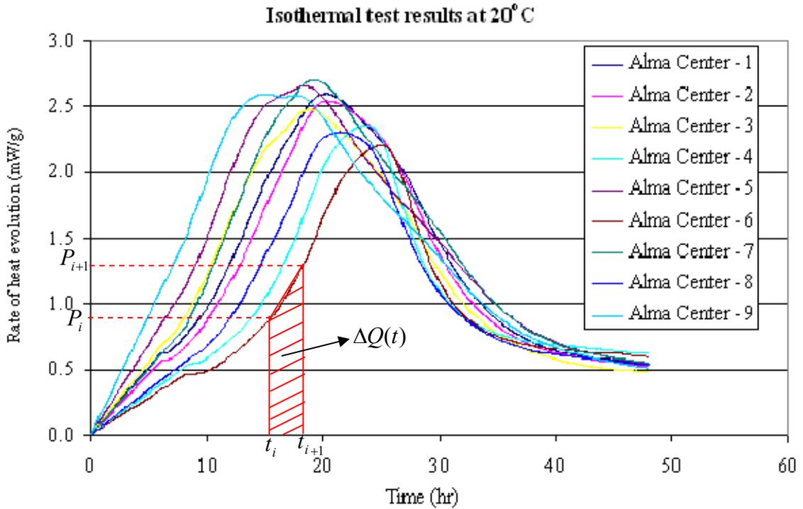
**Figure 76. Heat computation based on the trapezoidal method**
