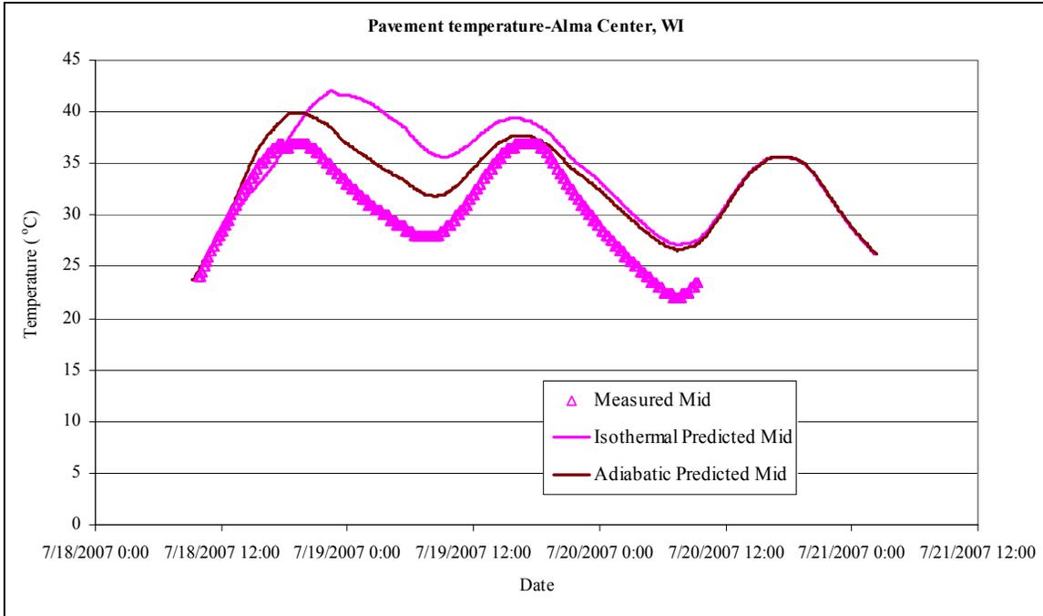
**Figure 99. Predicted pavement temperatures versus measurements (pavement mid, Alma Center, WI)**
