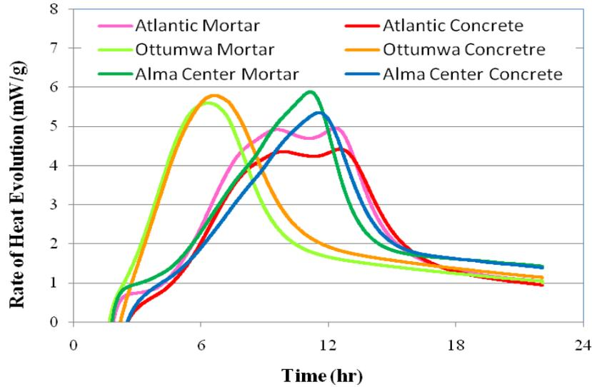
**Figure 28. Summary of isothermal field calorimetry results**
