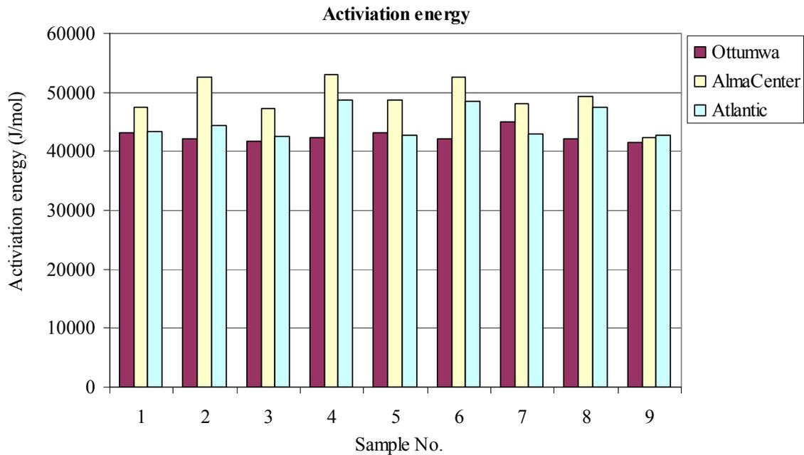
**Figure 71. Calculated activation energies for nine mixes at three sites based on the isothermal test results**
