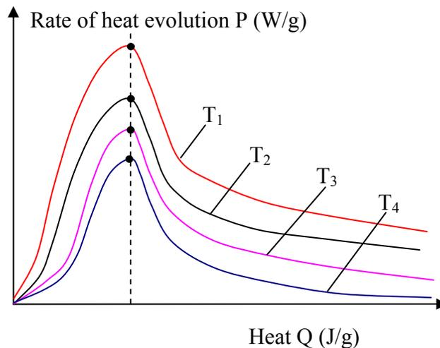
**Figure 66. Locate maximum hydration rate**
