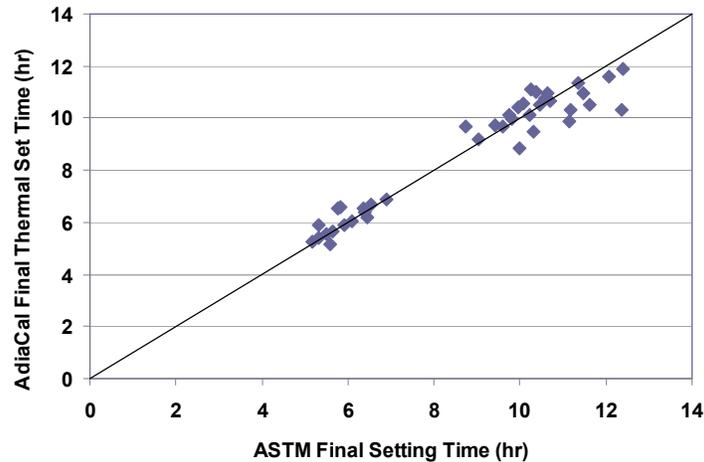
**Figure 27. ASTM set time vs. AdiaCal thermal set time—final set**
