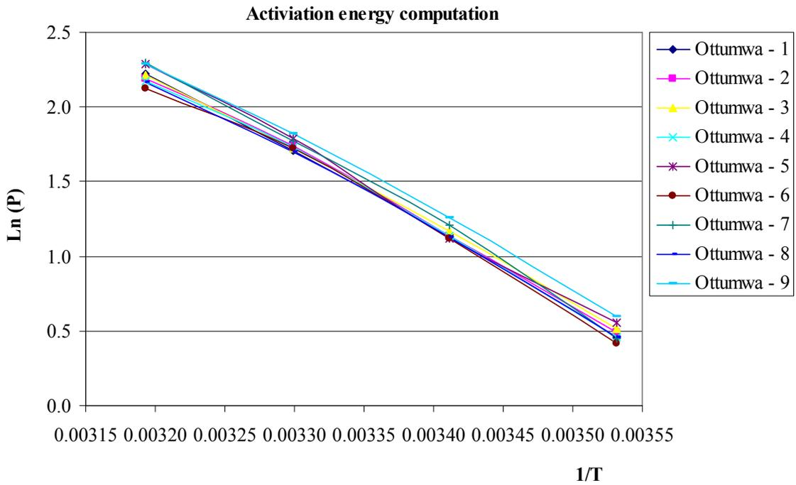
**Figure 70. Activation energy calculation for Ottumwa site (nine mixes, at four temperatures: 10 °C, 20 °C, 30 °C, and 40 °C; P unit: mW/g; T unit: K).**
