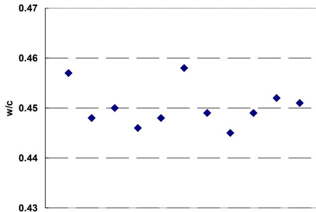
**Figure 14. Water to cement ratio for the mixes of HW 95 (Alma Center, WI) project**
