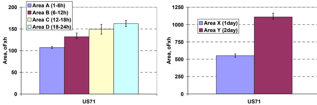
**Figure 32. Areas under AdiaCal test curves of US 71 (Atlantic, IA) project during different test period**
