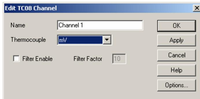
10. The Parameter options dialogue box is displayed. In the Units box, select mV. Input the desired numbers for the Number display and Scaling for graphs. Click OK twice until it goes back to the TC08 Channel dialogue box. Repeat the same procedure for the remaining channels. After defining all eight channels, click OK to accept all channels at the same time.
