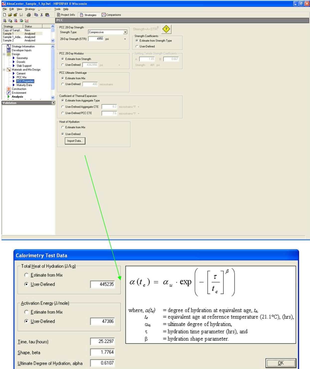
Figure 94. Windows of inputs of hydration curve parameters in the modified HIPERPAV II software.
