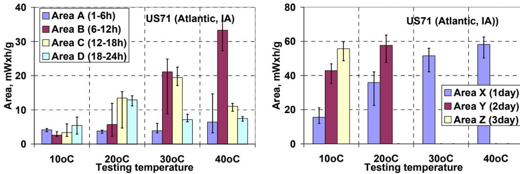
**Figure 37. Heat generation from isothermal robust test mixes at different times US 71 (Atlantic, IA) mixes**
