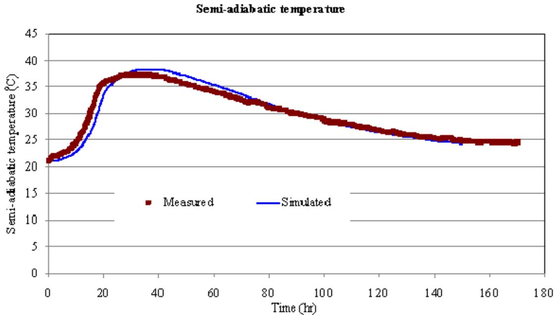
**Figure 92. Simulated semi-adiabatic temperature (from isothermal data) vs. measurements**
