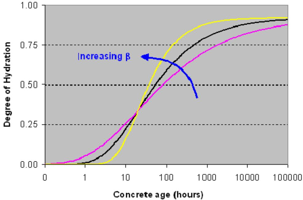
**Figure 74. Influence of hydration curve parameter  $\tau$  on degree of hydration**
