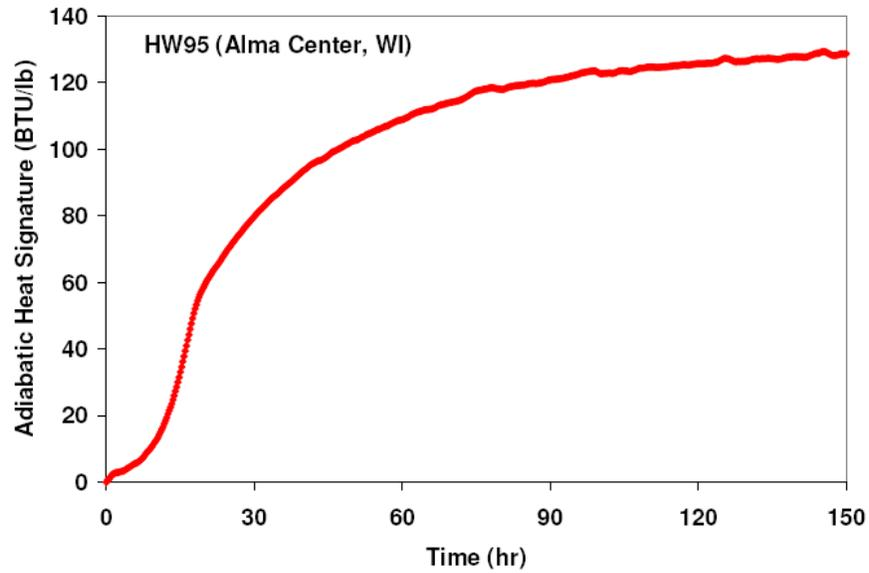
**Figure 50. IQ Drum test result of the HW 95 (Alma Center, WI) concrete (Mix 1)**
