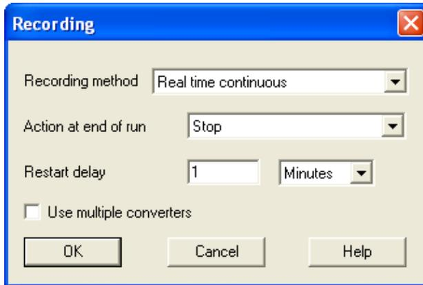
4. Select Real time continuous for Recording method. Define Stop as the Action at end of run and ignore other options, then press OK.
