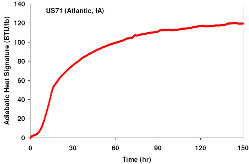
Figure 39. IQ drum test result of US 71 (Atlantic, IA) Mix 1
