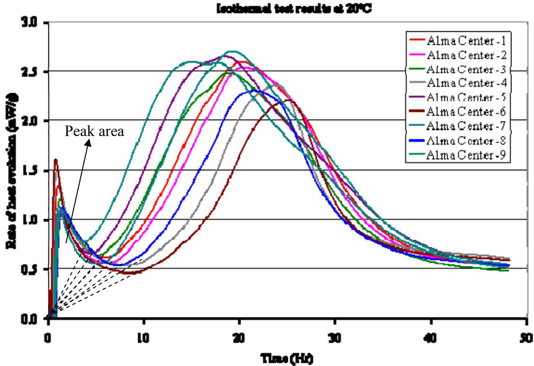
Figure 75. Pre-process the data of rate of heat evolution from isothermal tests
