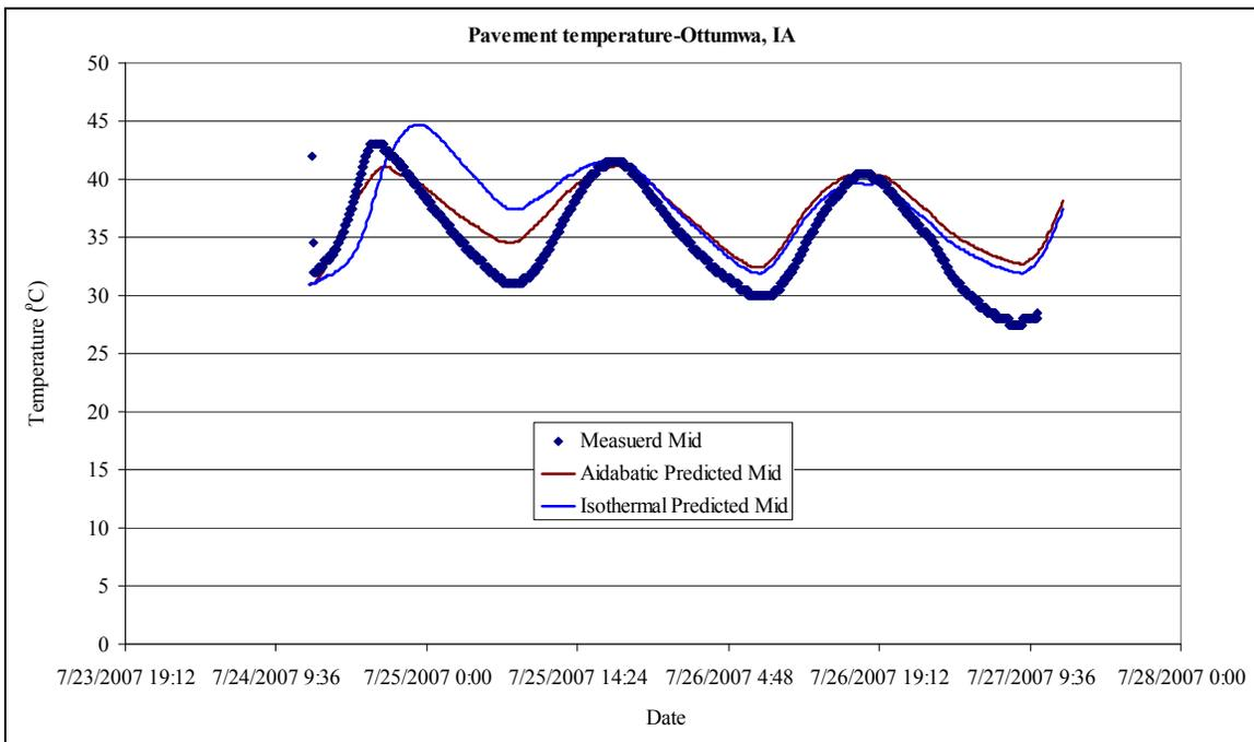
**Figure 111. Predicted pavement temperatures versus measurements (pavement mid, Ottumwa, IA)**
