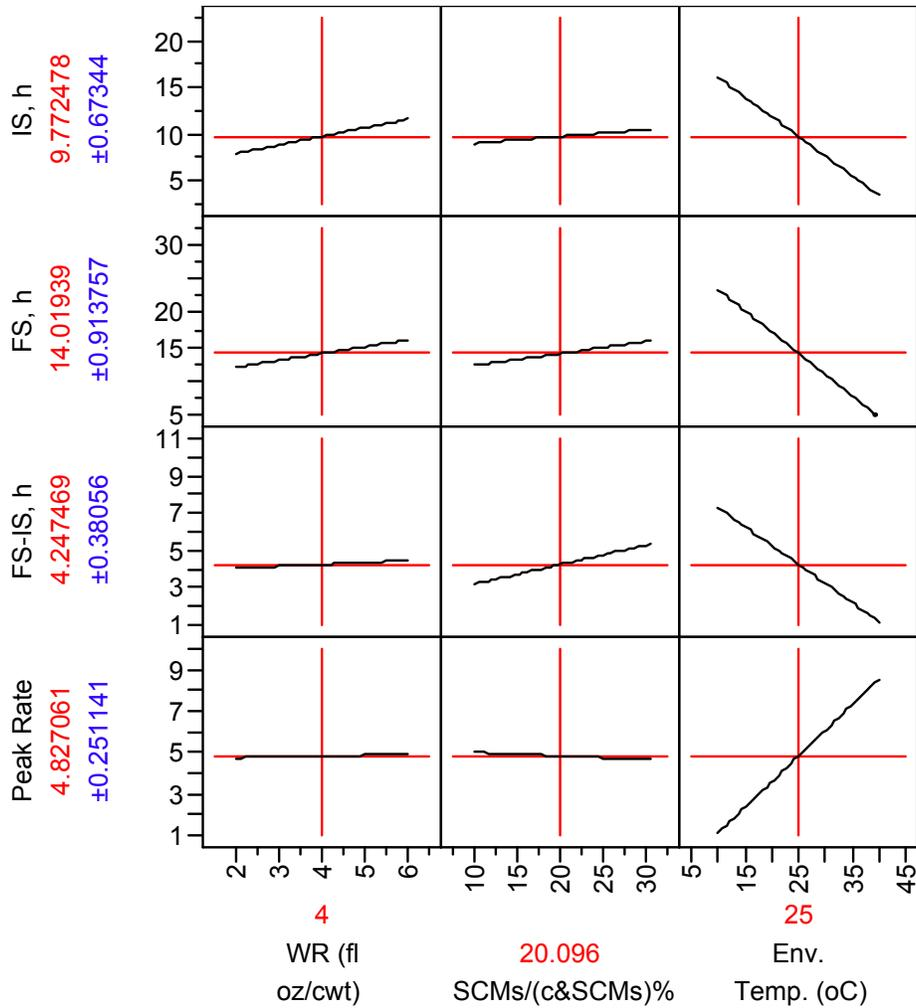
**Figure 59. Effect of mix design and temperature on IS and FS from isothermal robust test (US63 bypass (Ottumwa, IA) mixes)**
