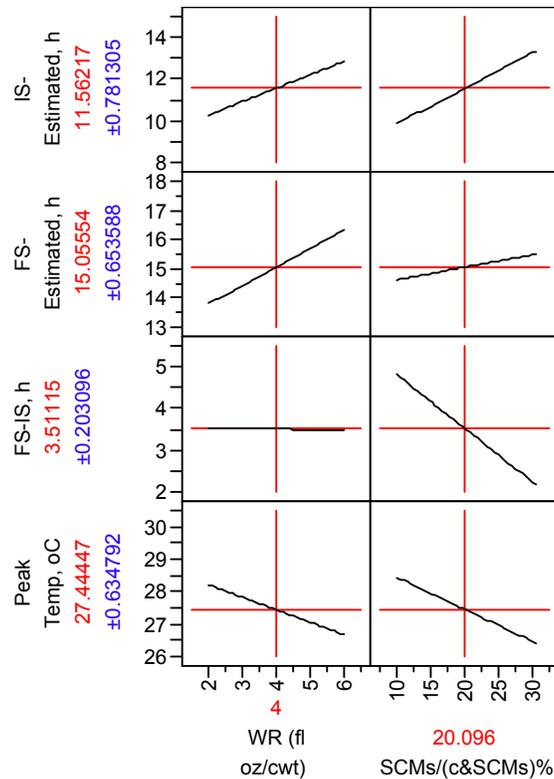
**Figure 54. Statistical analysis from the US 63 bypass (Ottumwa, IA) AdiaCal robust test**
