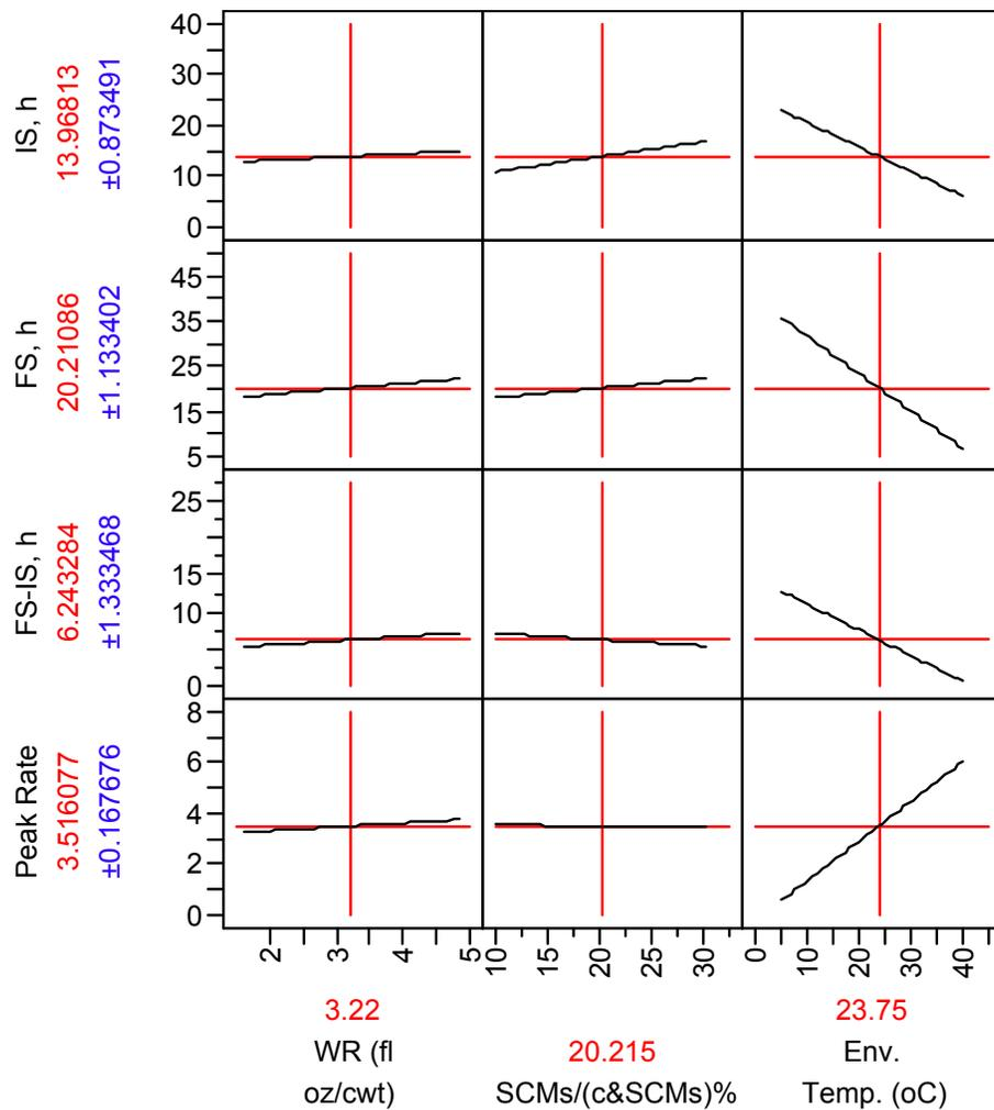
**Figure 48. Effect of mix design and temperature on IS and FS from isothermal robust test HW 95 (Alma Center, WI) mixes**
