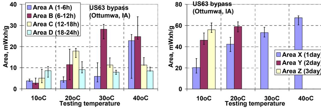
**Figure 58. Heat generation from isothermal robust test mixes at different times US 63 bypass (Ottumwa, IA) mixes**
