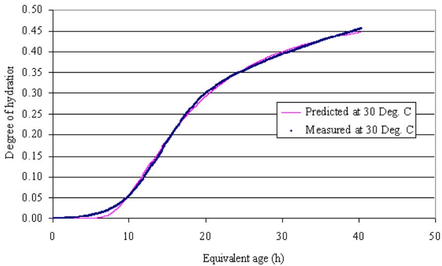
**Figure 79. Predicted degree of hydration vs. measurements at 30 °C (Sample 5, Alma Center)**
