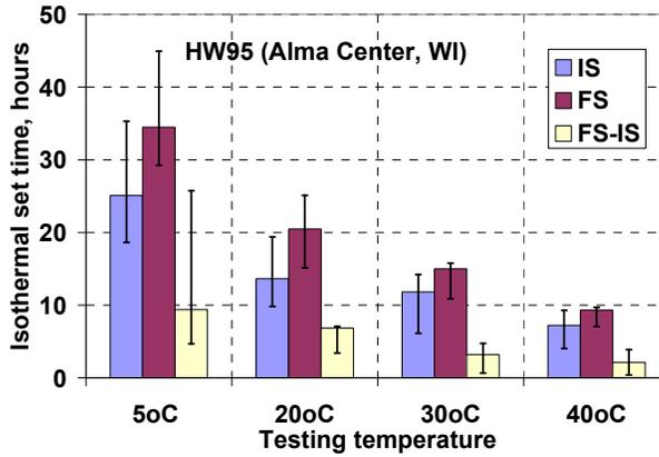
**Figure 46. Estimated set time from isothermal robust test on HW 95 (Alma Center, WI) mixes**
