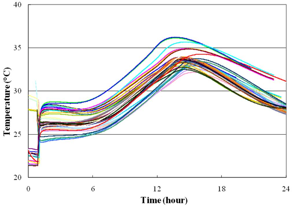
**Figure A.1. Concrete temperature for all samples for Atlantic project**
