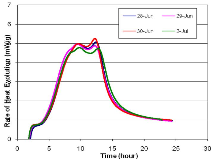
**Figure 8. Isothermal calorimetry results for US 71 (Atlantic, IA) field mortar samples**
