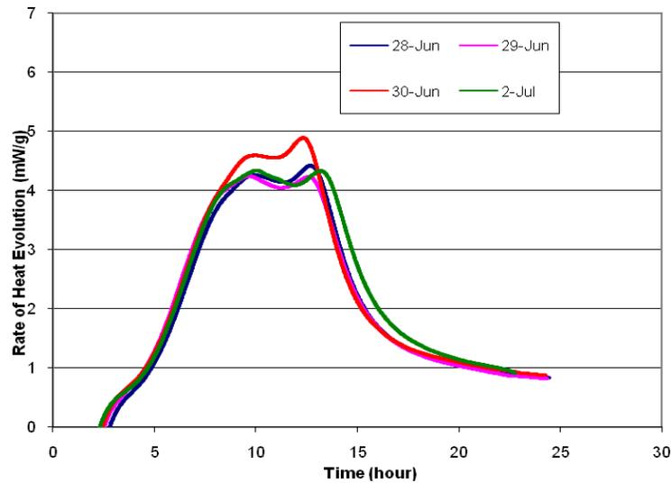
**Figure 9. Isothermal calorimetry results for US 71 (Atlantic, IA) field concrete samples**
