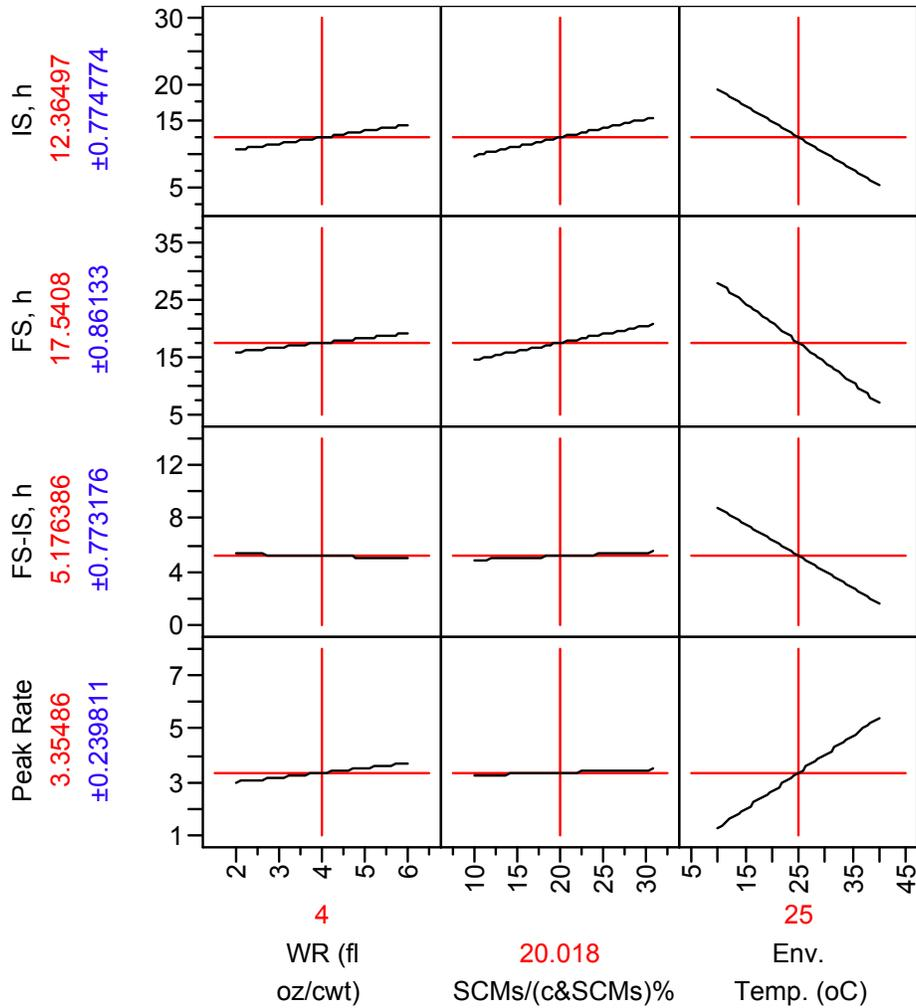
**Figure 38. Effect of mix design and temperature on IS and FS from isothermal robust test US 71 (Atlantic, IA mixes)**
