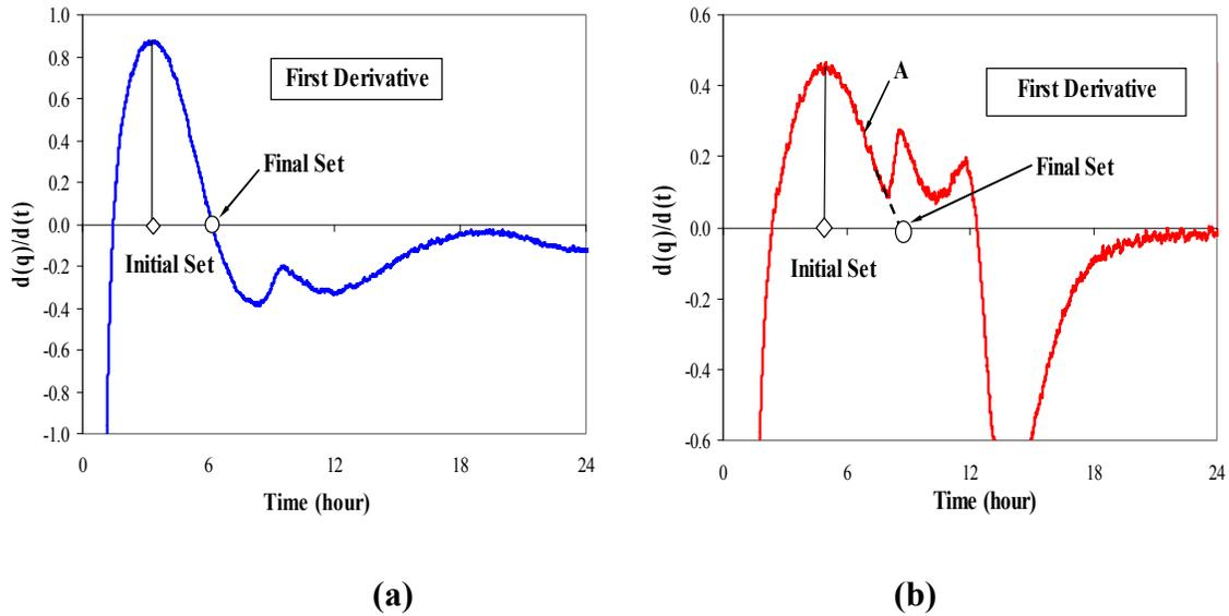
**Figure E.1. Determination of set times from heat evolution curve**
