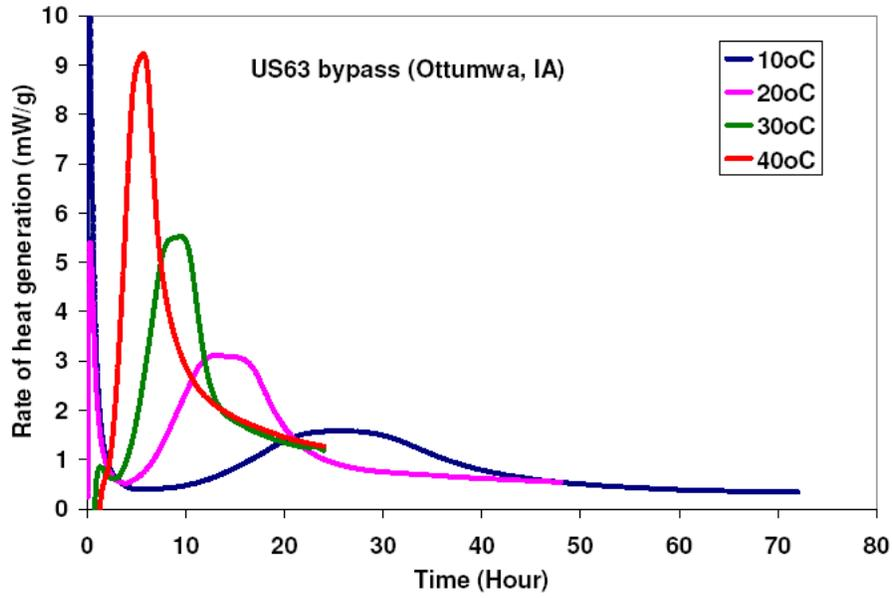
**Figure 55. Isothermal test results for US 63 bypass (Ottumwa, IA) mix 1 at different temperatures**
