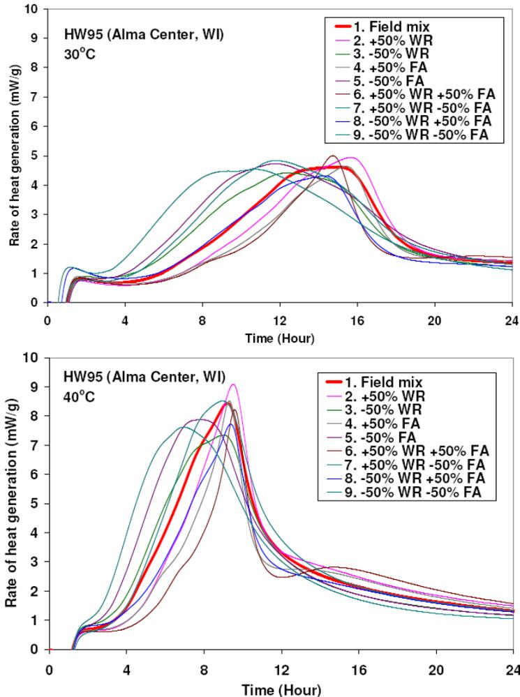
**Figure 45. Isothermal test results of HW 95 (Alma Center, WI) mortar mixes different temperatures**
