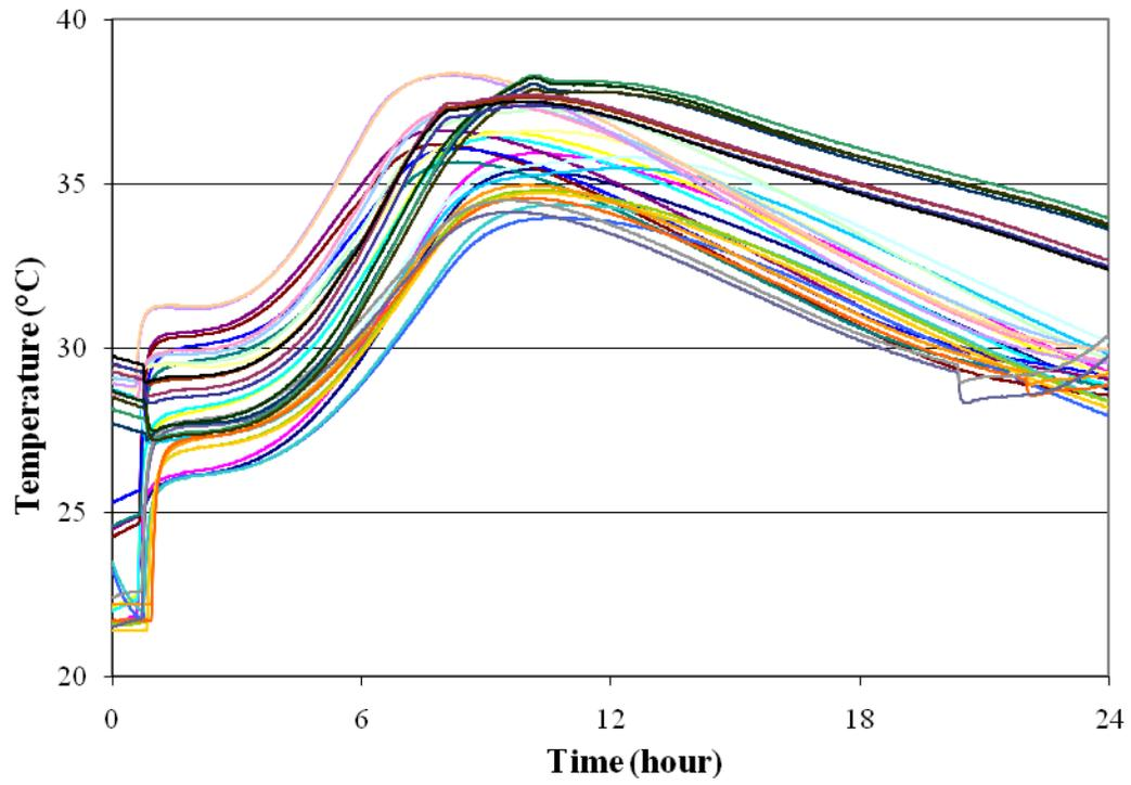
**Figure A.3. Concrete temperature for all samples for Ottumwa project**
