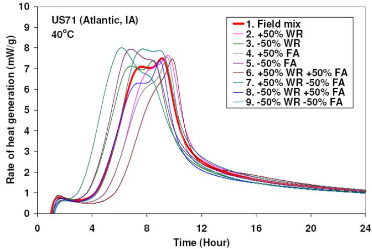
**Figure 35. Isothermal robust test results of US 71 (Atlantic, IA) mortar mixes at different temperatures**
