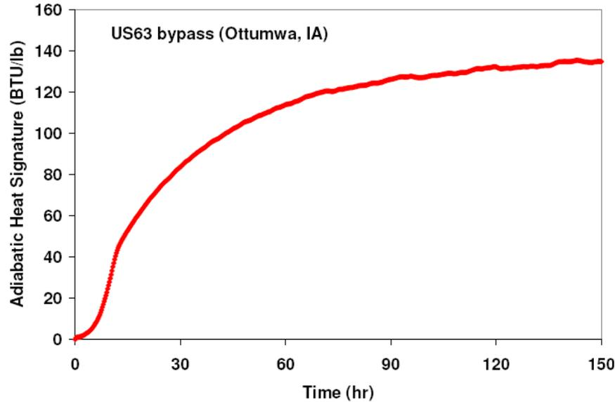
**Figure 60. IQ Drum test result of US 63 bypass (Ottumwa, IA) Mix 1**
