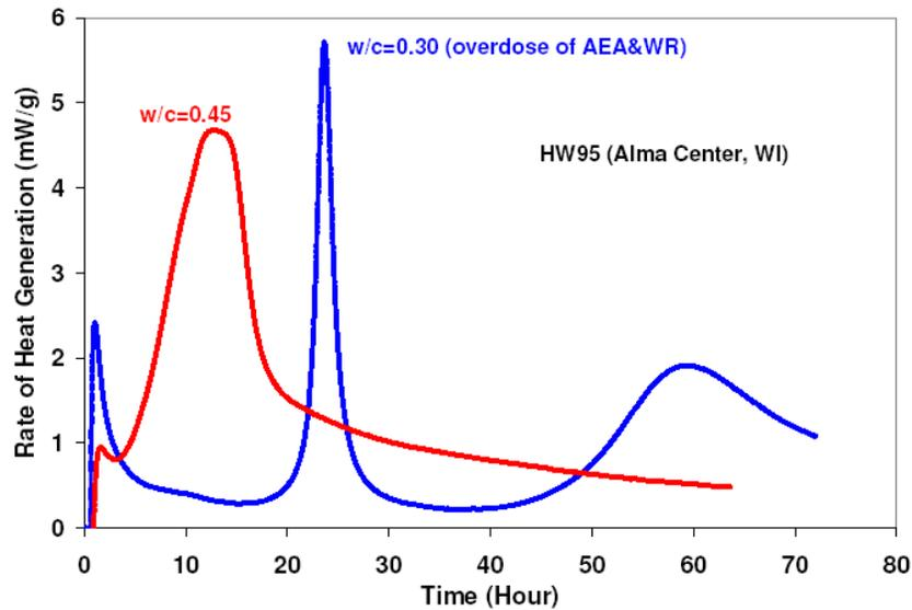
**Figure 49. Isothermal test results of mortar with normal and overdosed chemical admixtures**
