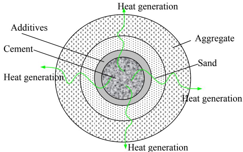
**Figure 91. Heat generation of cementitious material**
