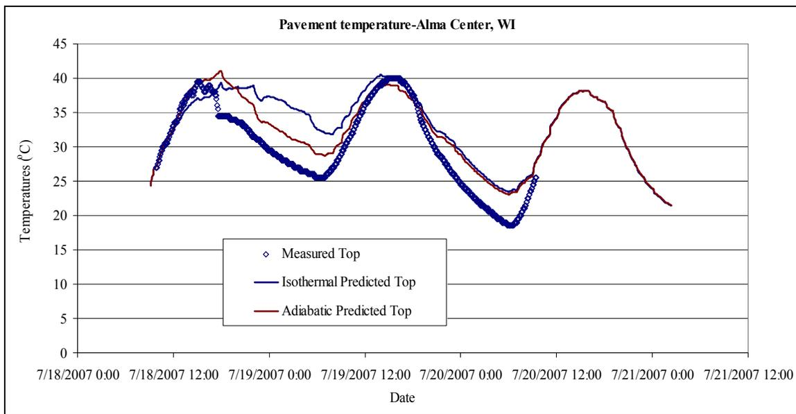
**Figure 98. Predicted pavement temperatures versus measurements (pavement top, Alma Center, WI)**
