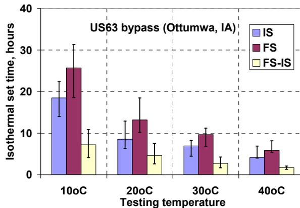
**Figure 57. Estimated set time from isothermal robust test on US 63 bypass (Ottumwa, IA) mixes**
