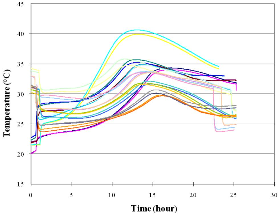
**Figure A.2. Concrete temperature for all samples for Alma Center project**
