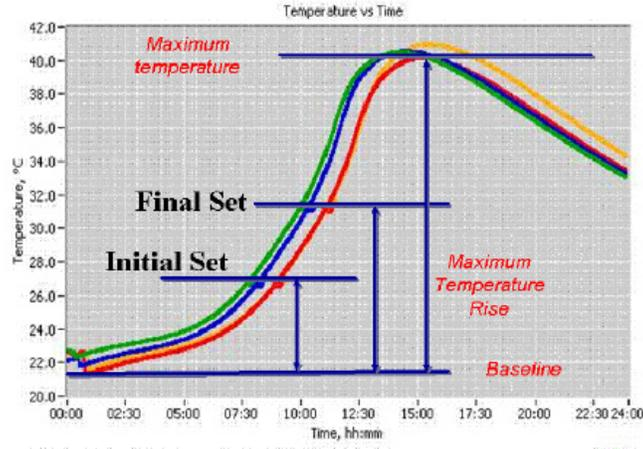
**Figure 6. AdiaCal test results and determination of the set times**
