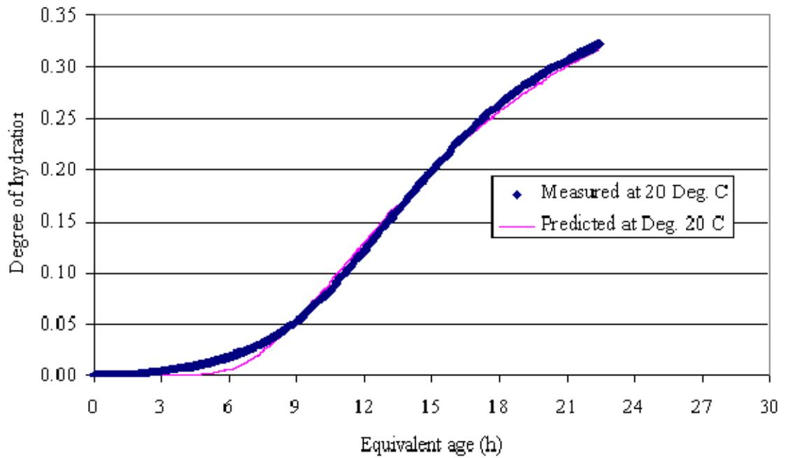
**Figure 78. Theoretical degree of hydration vs. measurements at 20 °C (Sample 5, Alma Center)**
