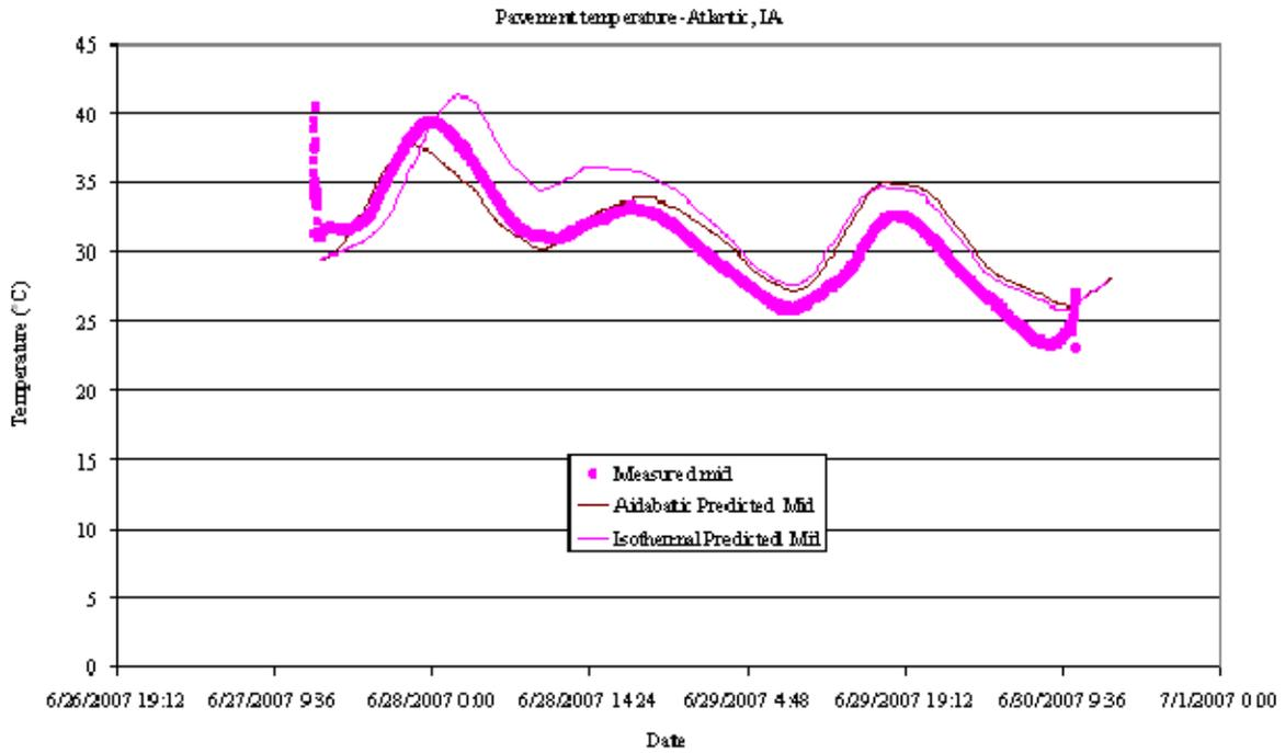
**Figure 105. Predicted pavement temperatures versus measurements (pavement mid, Atlantic, IA)**
