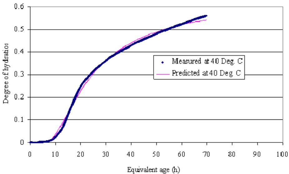
**Figure 80. Predicted degree of hydration vs. measurements at 40 °C for (Sample 5, Alma Center)**
