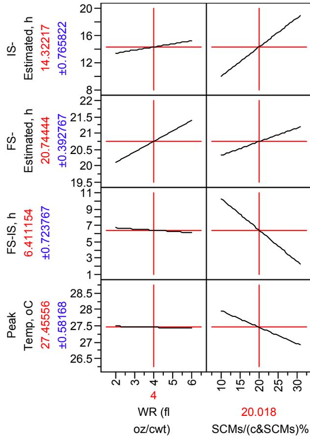
**Figure 33. Statistical analysis from US 71 (Atlantic, IA) AdiaCal robust test**
