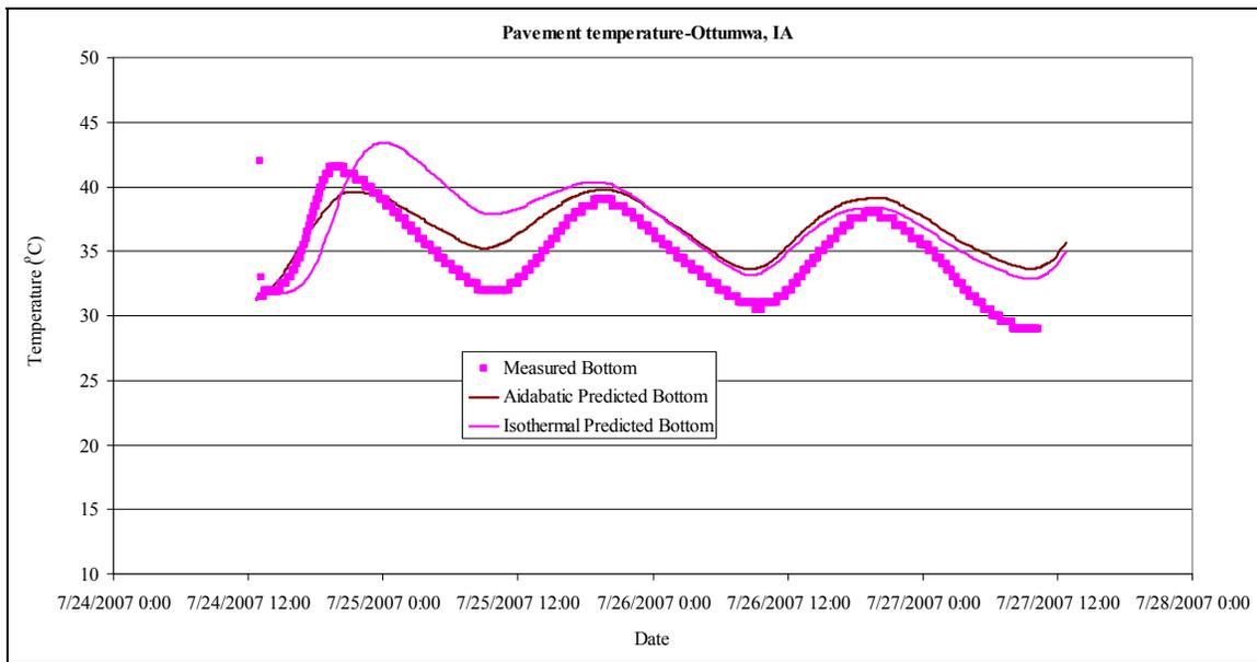
**Figure 112. Predicted pavement temperatures versus measurements (pavement bottom, Ottumwa, IA)**
