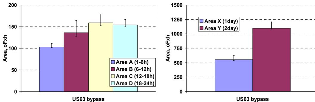
**Figure 53. Areas under AdiaCal test curves of US 63 bypass (Ottumwa, IA) projects during different test period**
