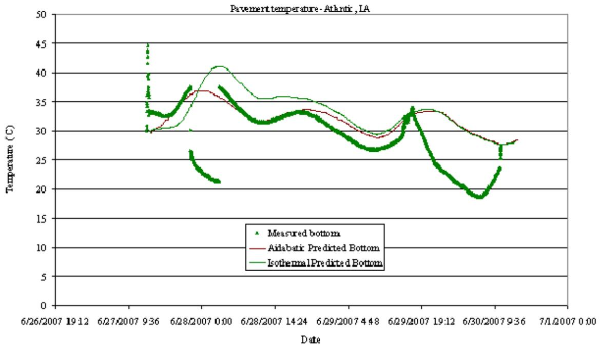
**Figure 106. Predicted pavement temperatures versus measurements (pavement mid, Atlantic, IA)**
