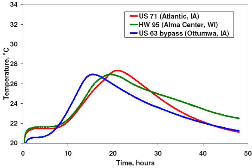
**Figure 62. AdiaCal calorimetry results from different projects (Mix 1)**
