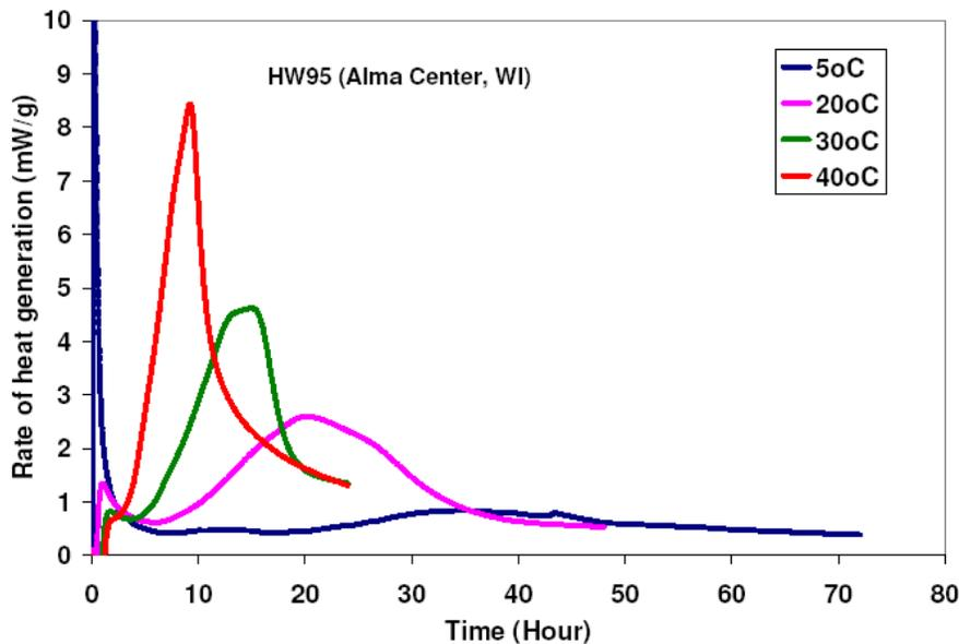
**Figure 44. Isothermal test results of HW 95 (Alma Center, WI) mortar mix 1 at different temperatures**
