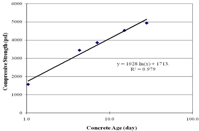
**Figure 19. Maturity-strength relationship for HW 95 (Alma Center, WI) samples**
