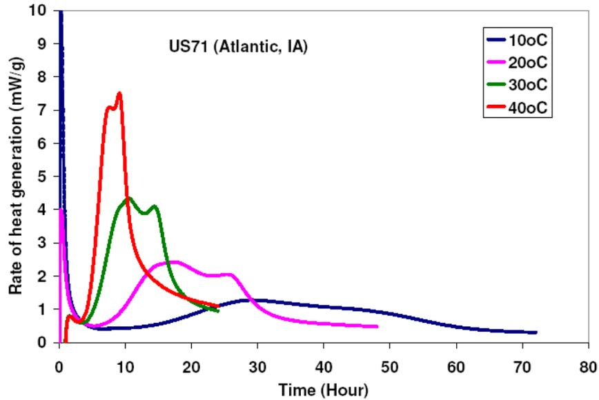
**Figure 34. Isothermal test results of US 71 (Atlantic, IA) Mix 1 at four temperatures**
