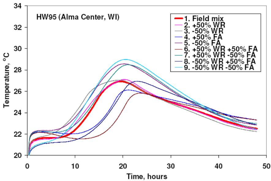
Figure 40. AdiaCal robust test results of HW 95 (Alma Center, WI) mortar mixes
