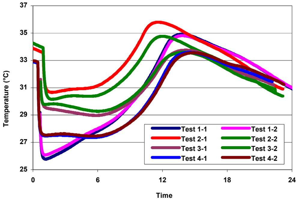
**Figure 16. Temperature from AdiaCal tests (tests were performed on HW 95, July 18<sup>th</sup>)**
