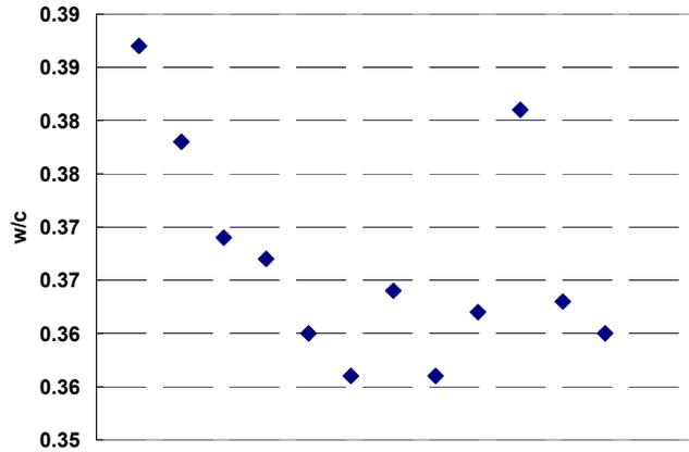
**Figure 21. Water to cement ratio for the mixes of US 63 bypass (Ottumwa, IA) project**
