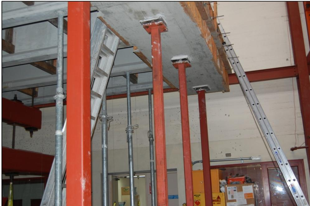
Figure 5.7: Temporary Support System Used Under Each Abutment
