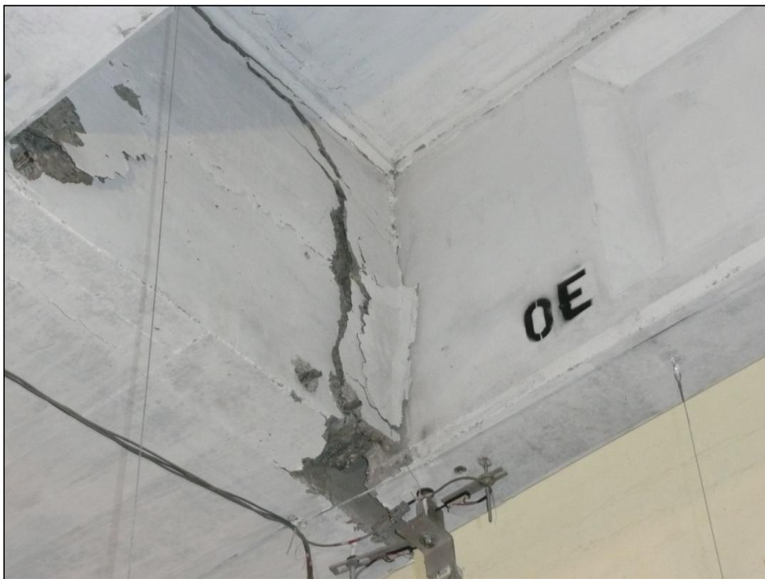
Figure 6.35: Damage to As-built Connection Exterior Girder at +2 in. Displacement
