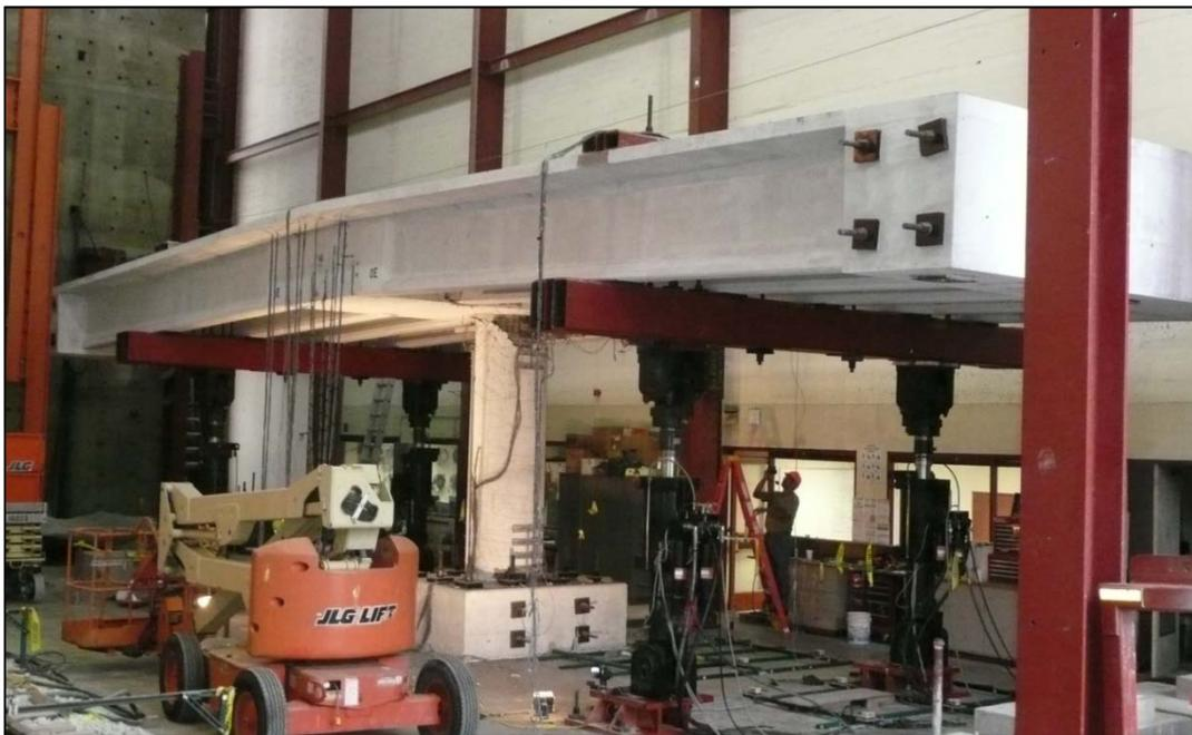
Figure 6.36: Displaced Test Unit at -6 in. of Displacement
