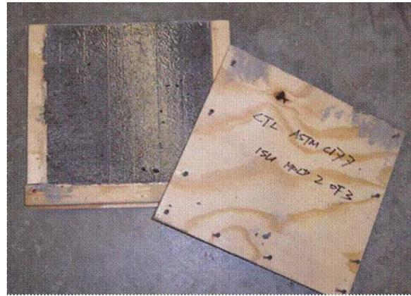
*Mold for PCC thermal conductivity samples*
