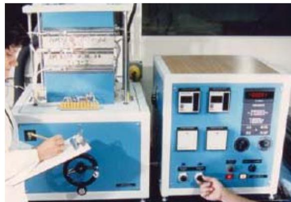
*Test setup for thermal conductivity*
