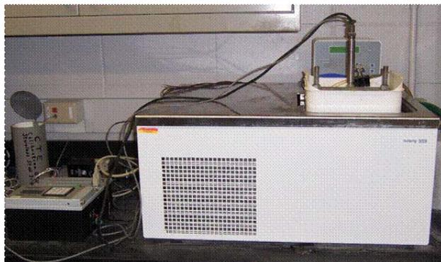
Test setup for measuring coefficient of thermal expansion
