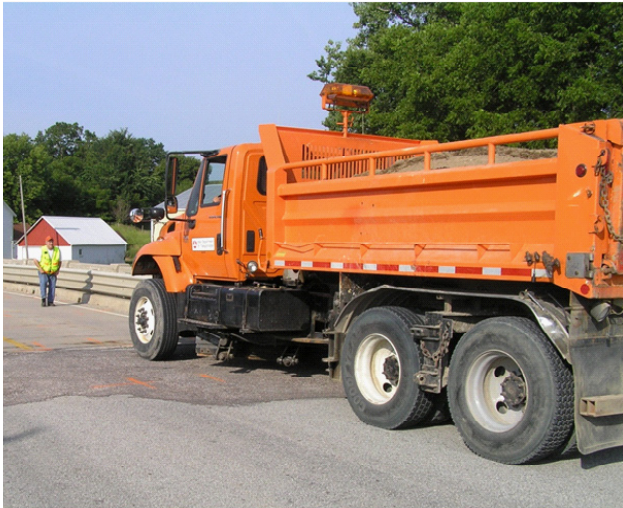
Positioning of load truck for static load test
